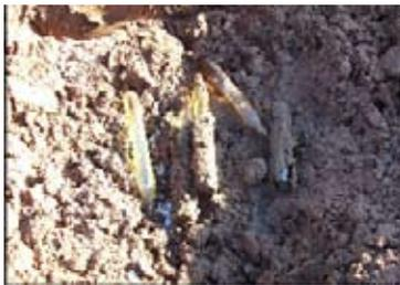
CAIS were either buried in their original metal or wooden storage and shipping containers — called Pigs — or loose. Normally, CAIS vials were broken before burial and the contents were neutralized. Because burial was one of the standard and approved procedures for disposing of CAIS, the possibility remains that buried CAIS may be discovered at active and former military installations.
