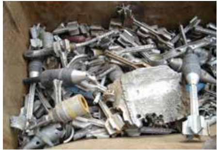
Mixed metals containing material potentially presenting an explosive hazard.
