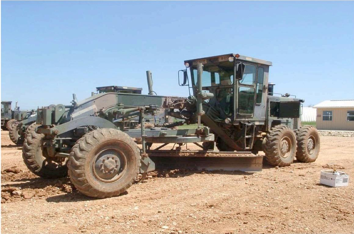
***The base's grader operates with biobased hydraulic fluid.***
