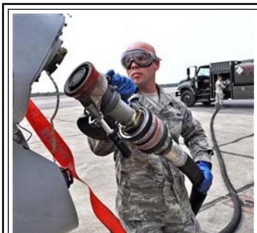
*Air Force Staff Sgt. Rusty Jones prepares to fuel an A-10C Thunderbolt II with a 50/50 blend of synthetic fuel and JP-8 at Eglin Air Force Base, Fla., March 25, 2010. The A-10 then flew the first flight of an aircraft powered solely by a biomass-derived jet fuel blend. U.S. Air Force photo by Samuel King Jr.*
