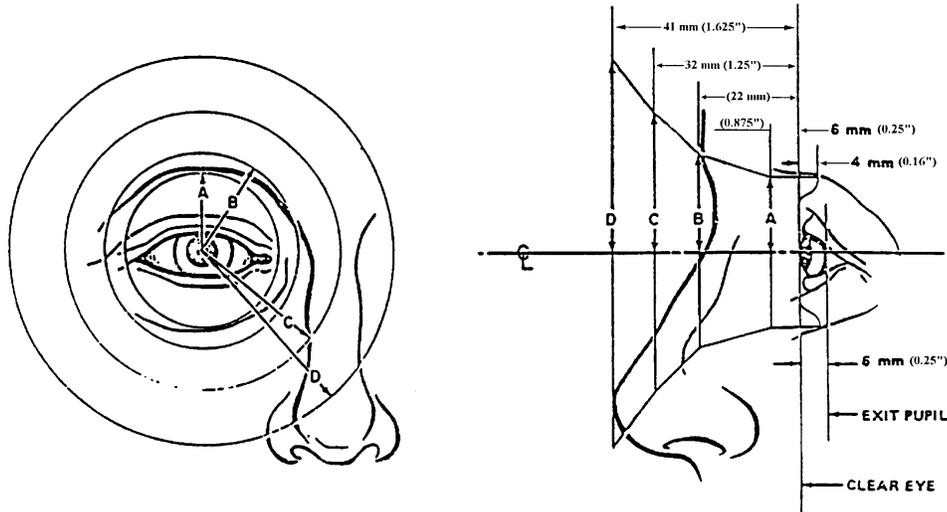
FIGURE 43. Anatomical limits on axially symmetrical ocular metal parts
