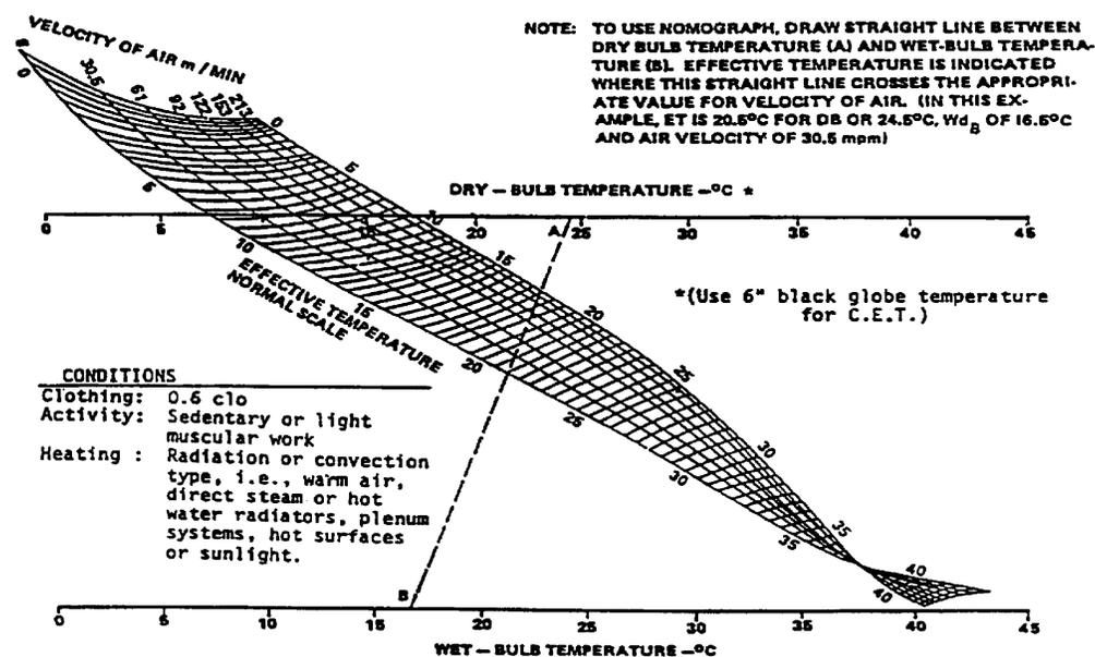
FIGURE 34. Effective temperature (E.T.) or corrected effective temperature (C.E.T.)
