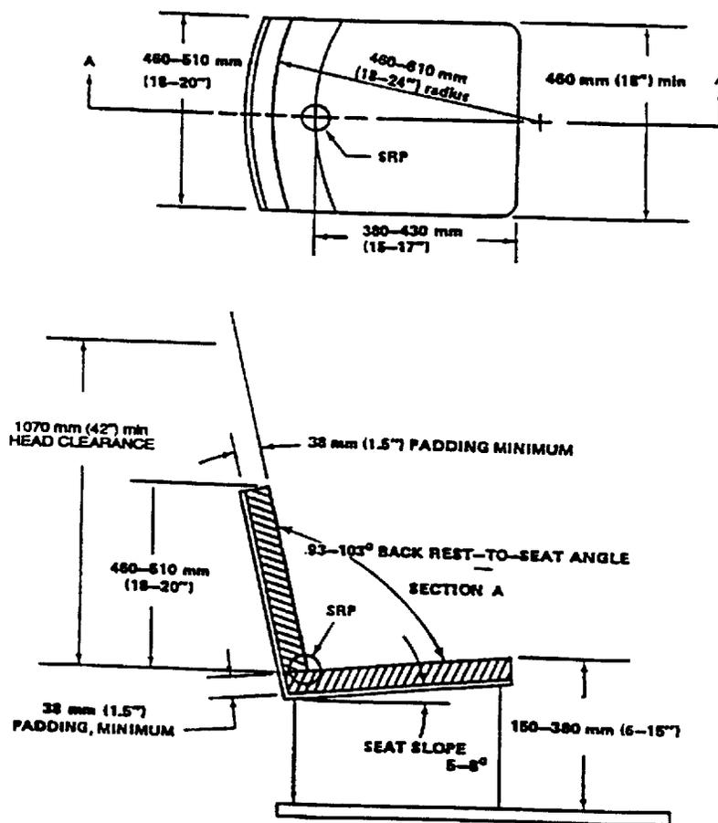
FIGURE 44. Dimensions for vehicle operator's seat
