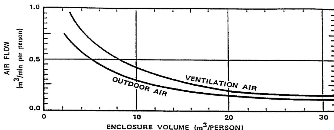
FIGURE 35. Ventilation requirements
