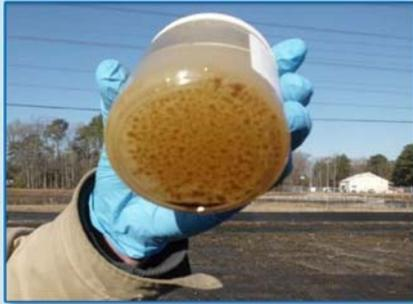
*Figure 4 – Dense Non-aqueous Phase Liquid from Site 2*
