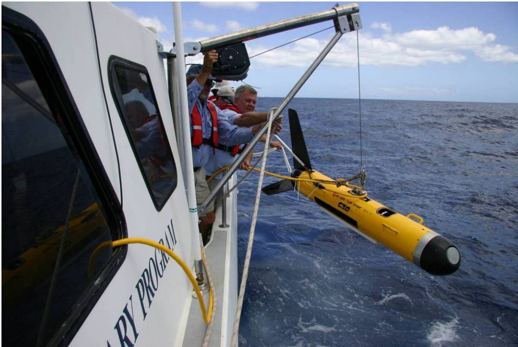
Figure 26. Teledyne Benthos C3D side scan sonar.
