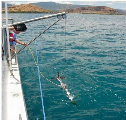
Figure 30. Teledyne Benthos 1624 side scan sonar
