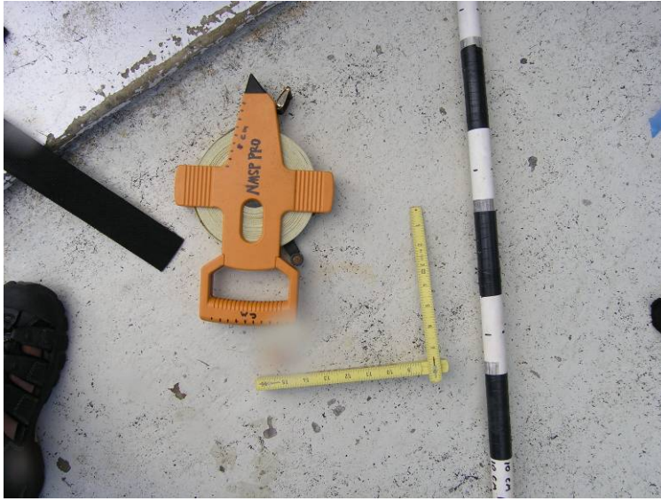
Figure 20. Diver measurement tools (black and white PVC scale used in photos in 10cm sections).
