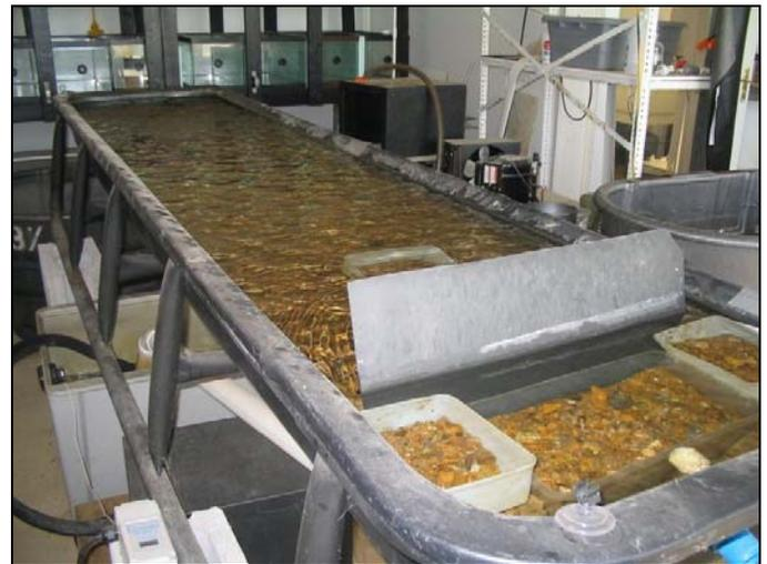
This is a model of a living stream, used to hold mature mussels until release. Water is pumped in from one end and drained out the other to emulate stream flow.
