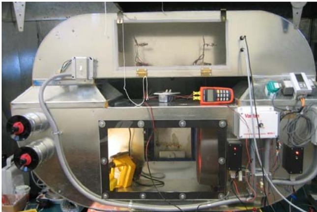
The climate controlled wind tunnel used to test ignition probability.
