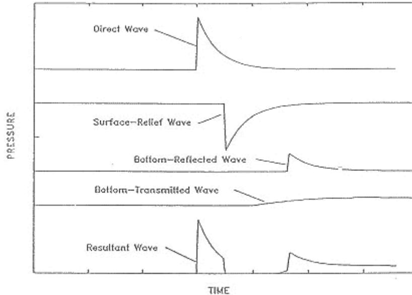
Figure 2.1. Shock-wave components and resultant wave (USACE, 1991)
