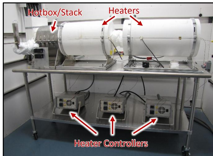
SOFC Stack Testing Apparatus
