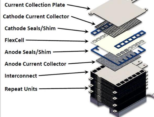
Expanded View of SOFC Stack
