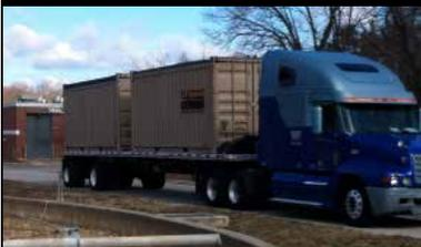
The wastewater treatment system is containerized for easy transport.
