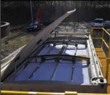
The AX-Mobile system features textile sheets in a packed bed media filter.
