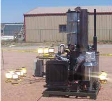
*A small-scale WTE system powers lights using wood chips and refuse-derived fuel, representative of solid waste generated in theater.*
