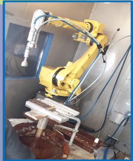
Example of a robotic water jet arm that is being used in our comparison testing
