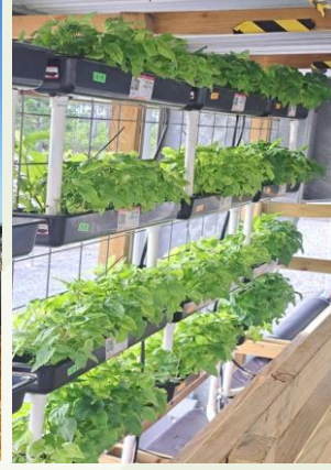
Lizard's tail plants in hydroponic system circulating wastewater from firefighter test operations. The water quality and PFAS sequestration monitored.
