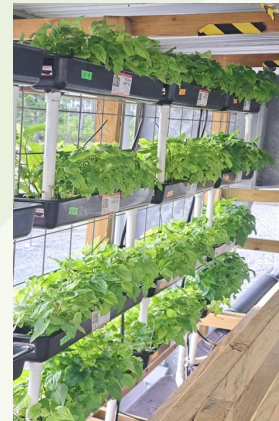
Lizard's tail plants in hydroponic system circulating wastewater from firefighter test operations. The water quality is monitored regularly and PFAS sequestration determined at end of trial.
