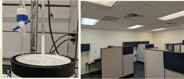
Water-based acrylic paint being treated with anti-mold additive at bench scale (left) and tested in a newly renovated office Tyndall AFB (right)
