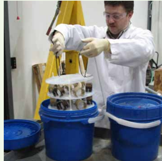
The NDCEE investigated whether cleaning solutions contributed to hydrogen embrittlement in high strength steel. Results may allow Corpus Christi Army Depot, TX, to optimize its maintenance processes.
