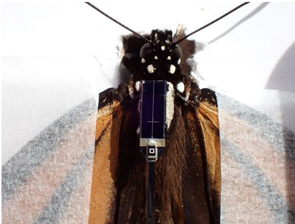
Image of CTT BluMorpho tag attached to the dorsal thorax of a monarch butterfly. Glassine envelopes cover the wings to minimize scale loss during handling. Photo courtesy of Kyle Nessen, Cal Poly/Althouse & Meade.
