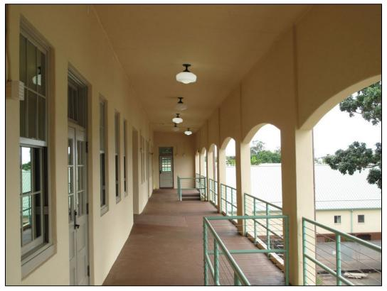
Figure 4. Building 690 showing large windows and balconies for airflow, 2015 (US Army Garrison-Hawaii).
