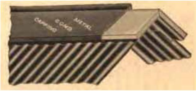
*Illustration 12: Corrugated metal roofs required a cap along the ridge (Globe Iron and Corrugating Company 1890:25-26).*
