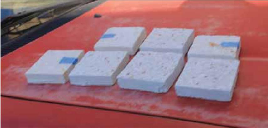
*Illustration 65: The concrete mock-ups for the patching to Building 3. Each sample varies slightly in color and/or aggregate type (Photographer: Samantha Driscoll 2015).*
