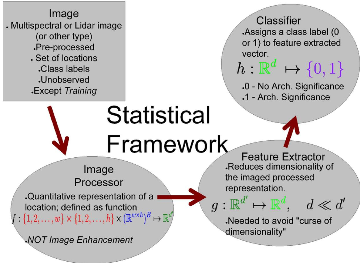
Figure 11: Schematic of Statistical Framework
