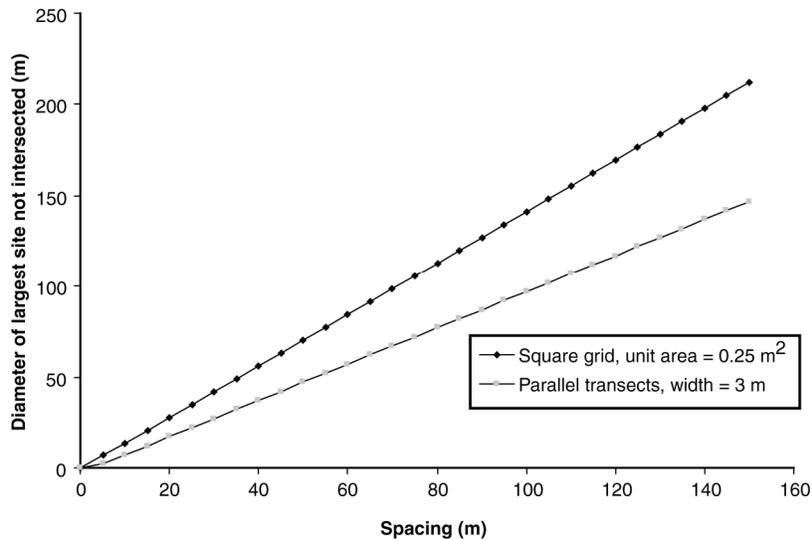
**Figure 2.6. Comparison of the largest site not intersected for square grids and pedestrian transects, according to spacing.**
