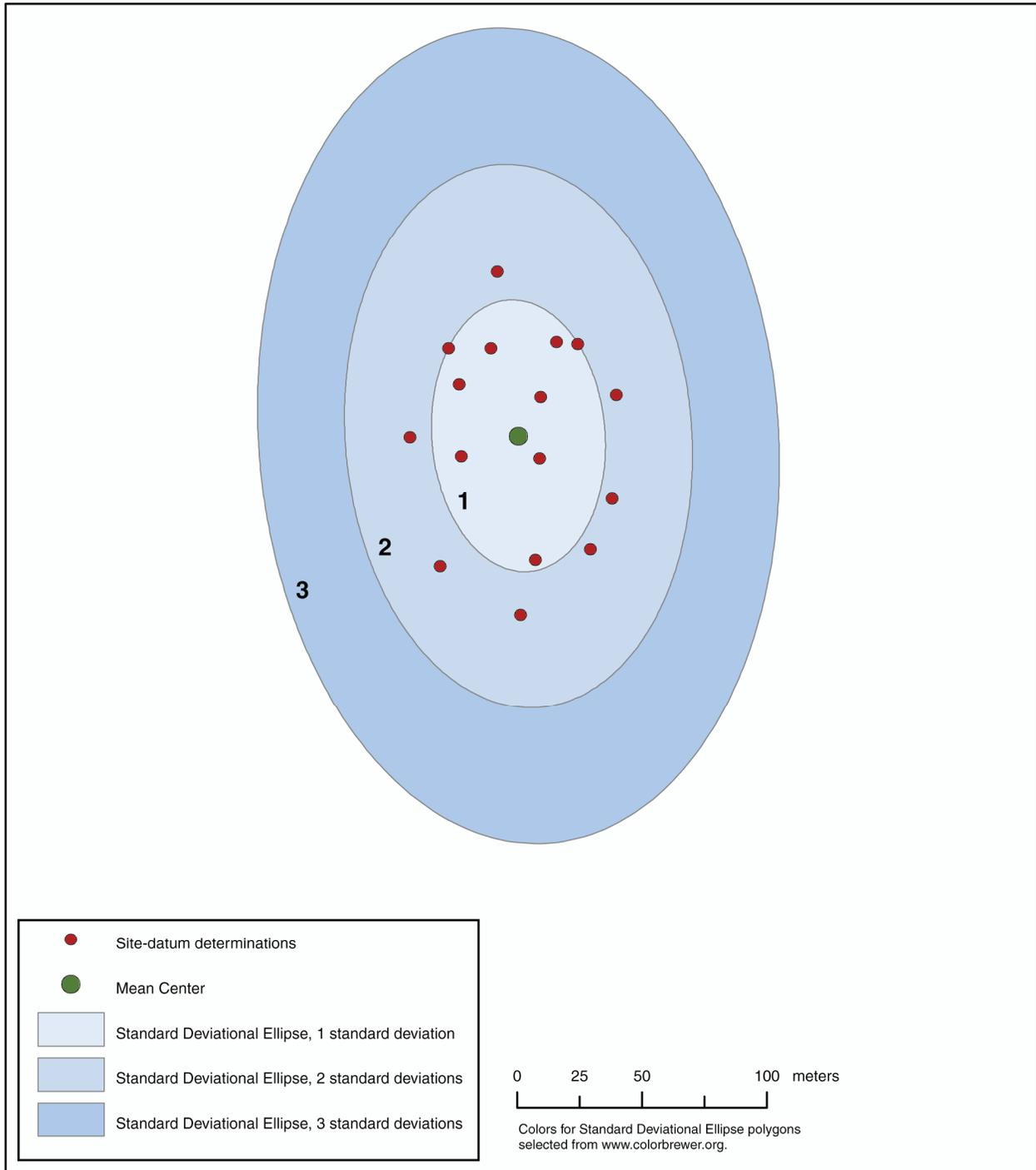
**Figure 3.14. Hypothetical site-datum points (including outliers), determined over time by GPS, showing positions of Mean Center and Standard Deviation Ellipses for 1, 2, and 3 standard deviations.**
