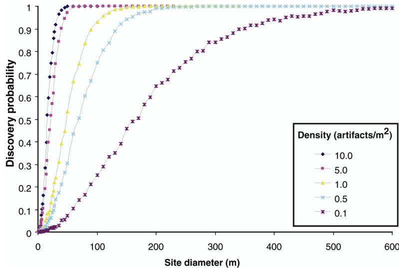
**Figure 2.19. The probability of discovery for 15-m spacing on a square grid and 30-by-30-cm test units, according to artifact density and site size.**
