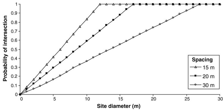
**Figure 2.3. The probability of intersection for 15-m, 20-m, and 30-m spacing, when transect width is 3 m.**
