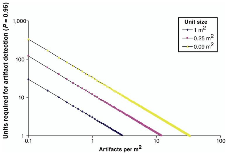
Figure 2.5. The number of units required to guarantee detection of at least one artifact for unit sizes of 0.09 m<sup>2</sup>, 0.25 m<sup>2</sup>, and 1.0 m<sup>2</sup> ( $P = 0.95$ ). Both scales are logarithmic.
