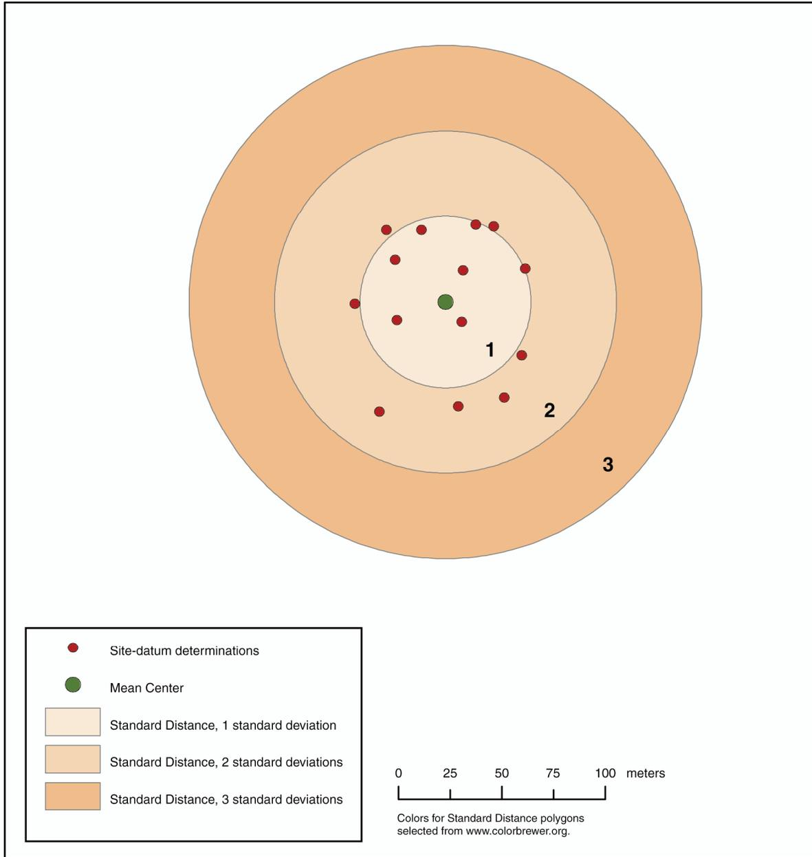
**Figure 3.17. The Standard Distance statistic (a circular polygon) for the hypothetical site-datum points (excluding outliers), describing the compactness of the distribution. Polygons for 1, 2, and 3 standard deviations are shown.**
