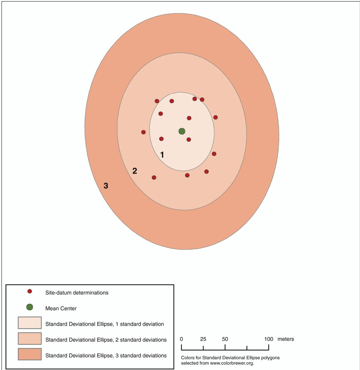
**Figure 3.15. Hypothetical site-datum points (excluding outliers), determined over time by GPS, showing positions of Mean Center and Standard Deviational Ellipses for 1, 2, and 3 standard deviations.**
