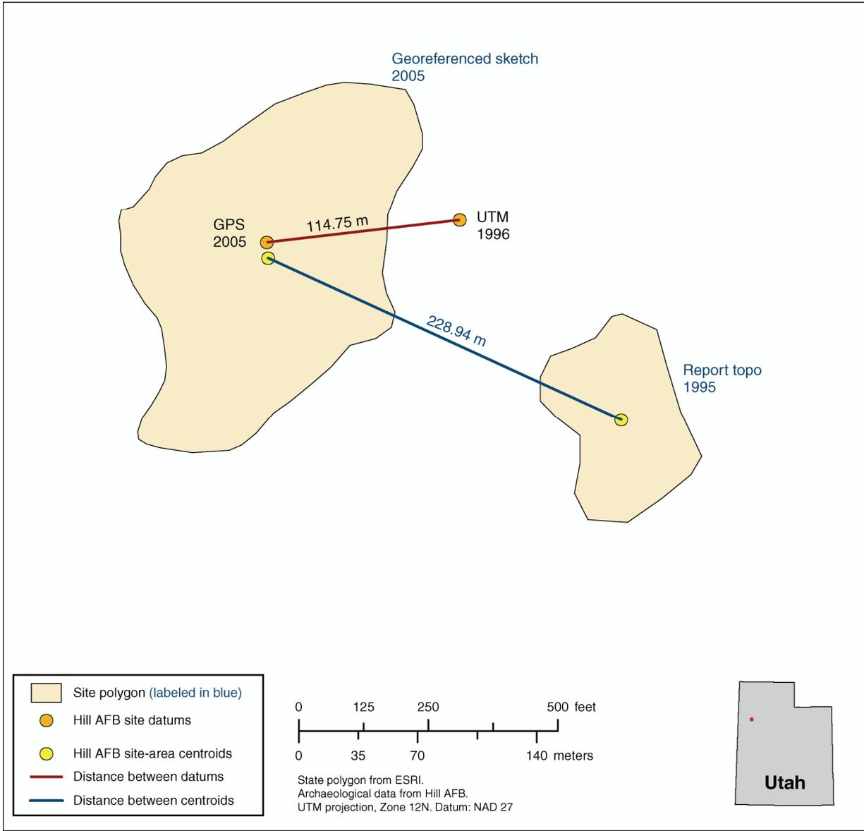
**Figure 3.12. Example of site-area change over time: site 42BO0911. This site has two site-datum points associated with two site-extent polygons.**
