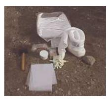
Spill Kits should be maintained in and around all locations where HM/HW are stored, handled or disposed of. Various types of kits can be ordered through the Army Supply System (see <u>Appendix B</u>) and should include: rubber gloves, safety goggles, putty, rubber mallet, wooden plugs, absorbent booms, absorbent pads, plastic bags, and in some cases a disposal barrel.
