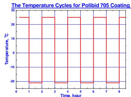
Fig.3. Temperature Cycles
