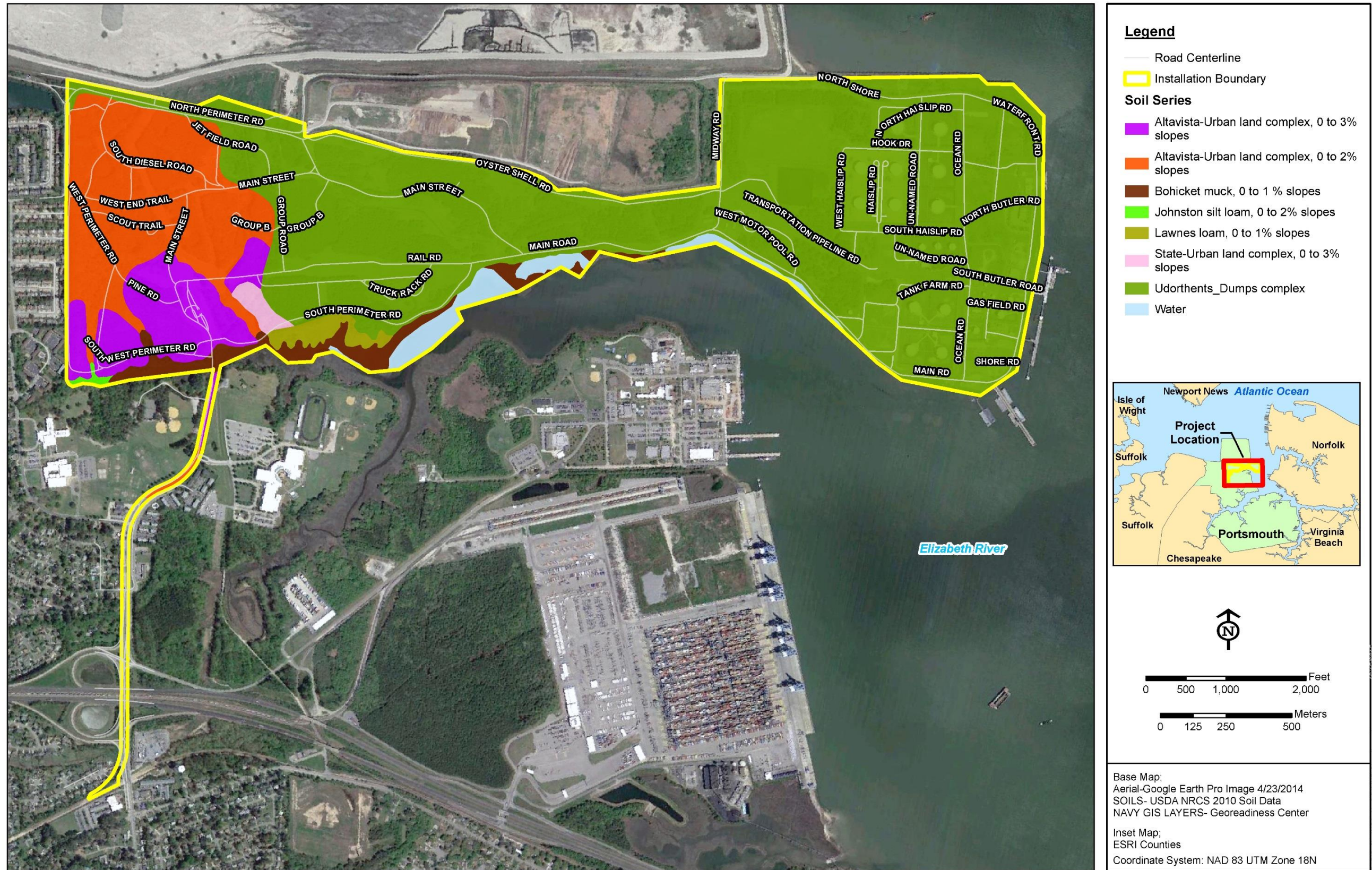
Figure 2-2. Soils of Craney Island Fuel Terminal, City of Portsmouth, Virginia.
