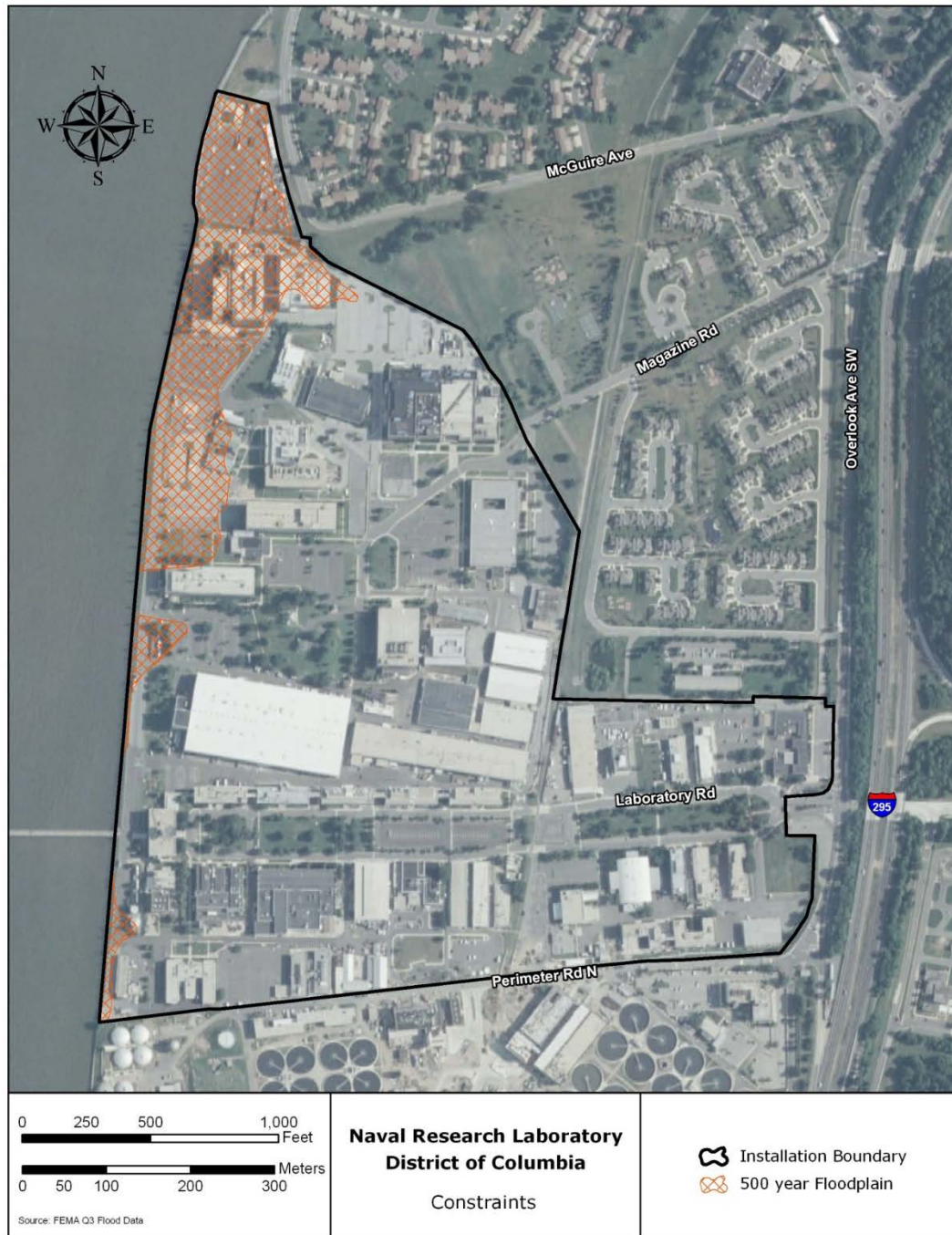
Figure 2.2. Constraints Map for NRL-DC. Potential constraints for NRL are a lack of undeveloped land and predominance of impervious surfaces; air quality; Potomac River water quality and aquatic biota; and a 38-acre 500-year flood along the Potomac River.
