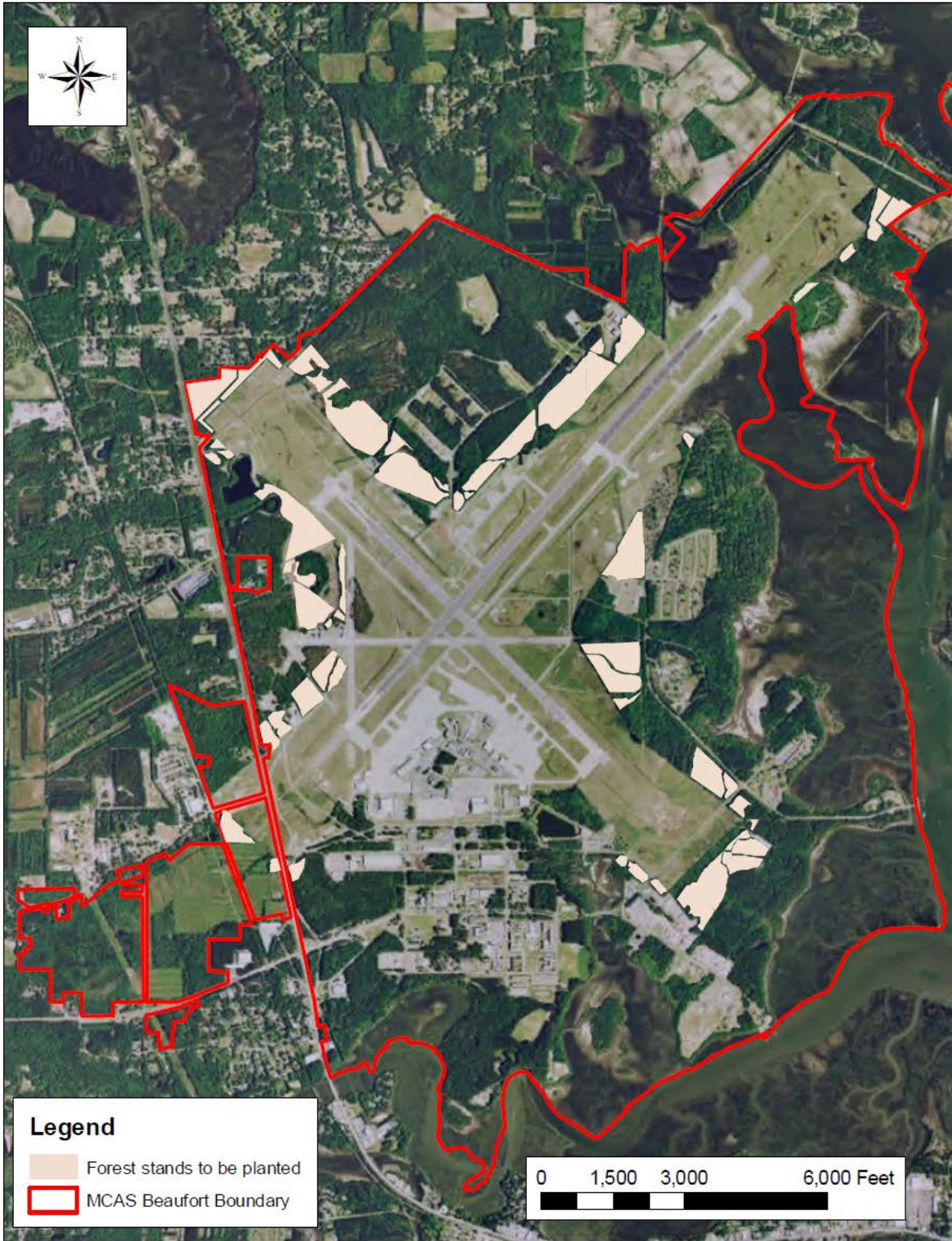
Figure D-4. Timber Areas Managed for Clear Zone Compliance and More Effective Aircraft-to-Ground Communications.
