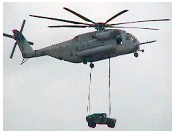
CH 53 lifting HMMWV
