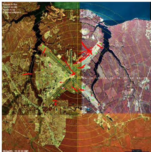
Accipiter® software demonstrates a single hour of bird movements around MCAS Cherry Point, with tracks clearly visible.
