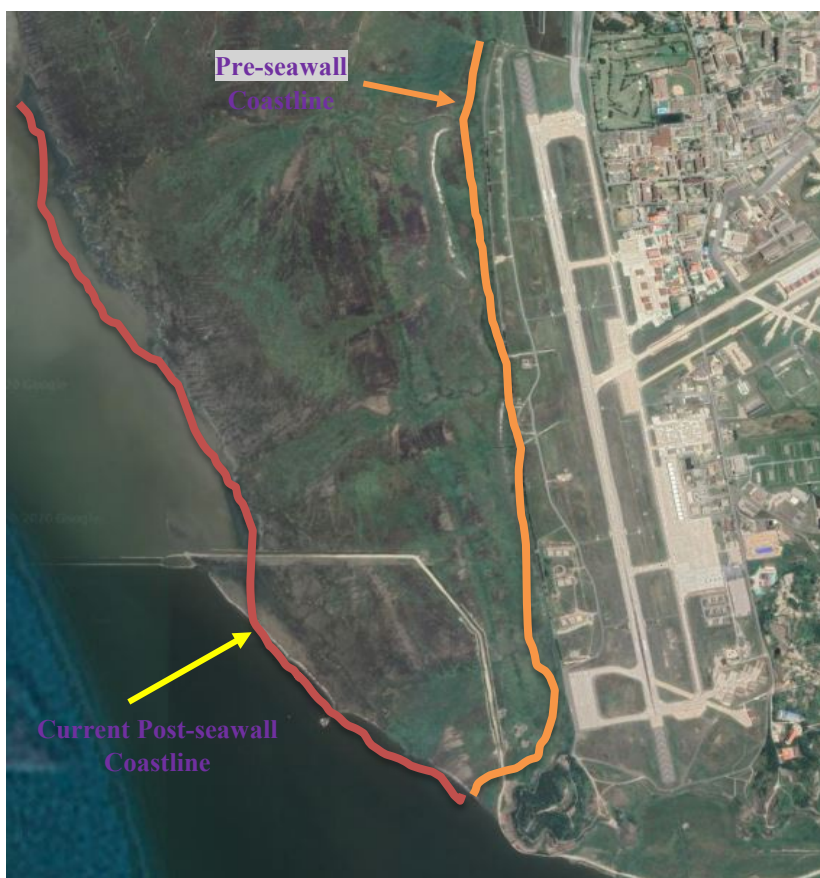
Figure 2.6 Yellow Sea Coastline Retreat at Kunsan AB following Completion of the Saemangeum Seawall, Present Day.
