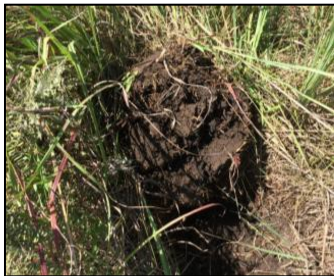
Figure 1-7: Typical soil at the KSTC has strong granular structure, with approximately 2 to 5 percent organic matter.
