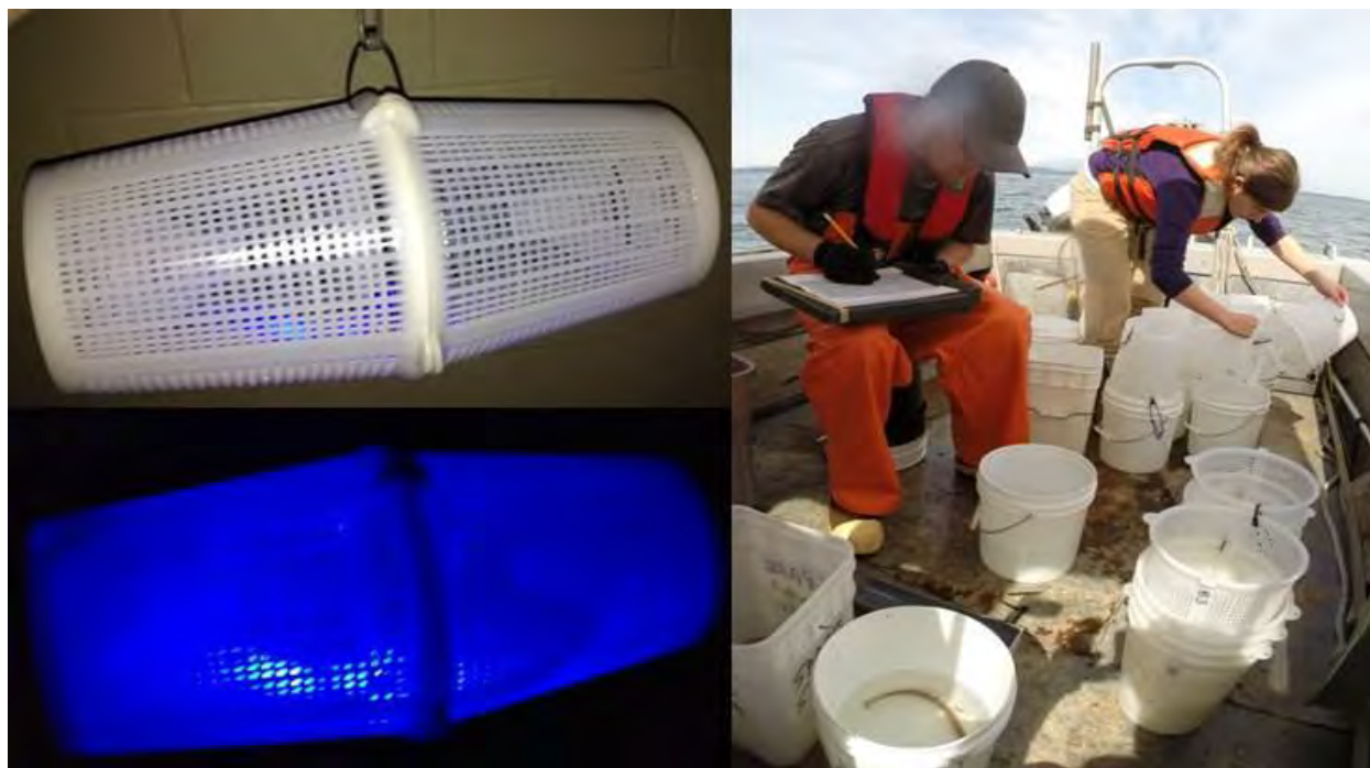
Figure 6. Lighted fish trap example showing single trap illuminated with blue LED (left). WDFW staff aboard a research vessel processing marine organisms captured in light traps (right).
