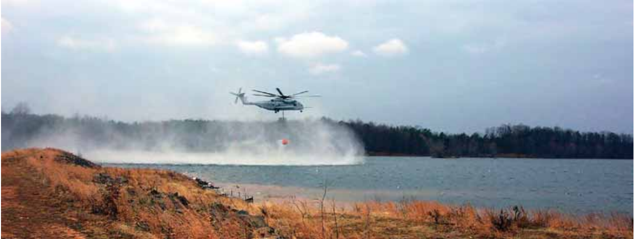
Figure 5-9. Valuable fire suppression support is provided by the HMX-1 Helicopter Squadron using a "Bambi Bucket" for water delivery.
