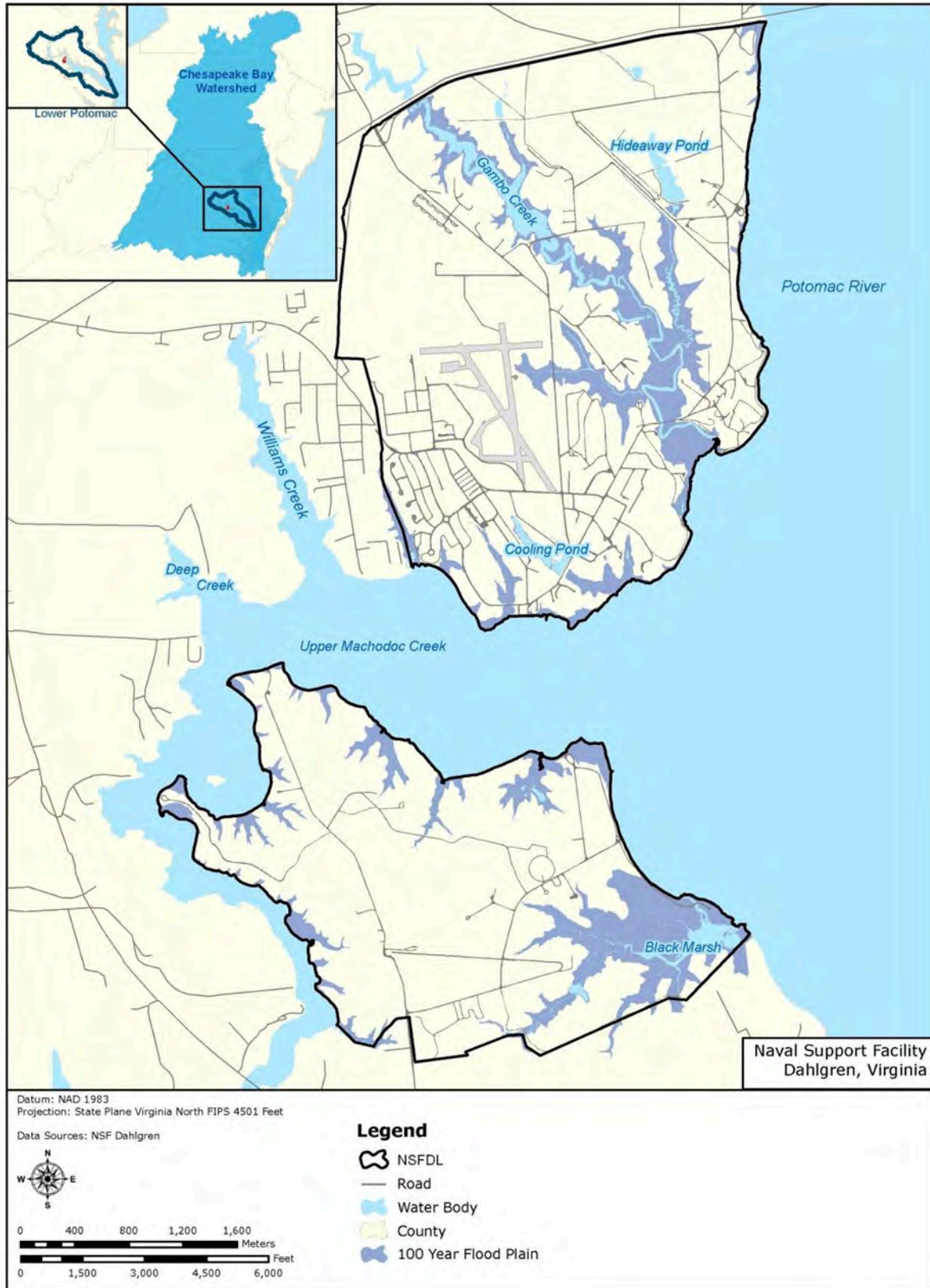
Figure 2-9. Naval Support Facility Dahlgren 100-Year Floodplain
