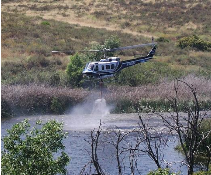
Photo 41. Helicopter refilling at Depot Lake for water drops during fire suppression. (Photo by C.M. Wolf)
