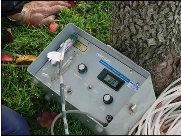
Fumiscopie for monitoring fumigant gas in structure.
