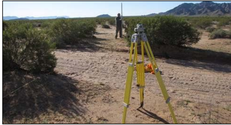
Figure 2.14: Measurements being taken using California rod and auto-level.
