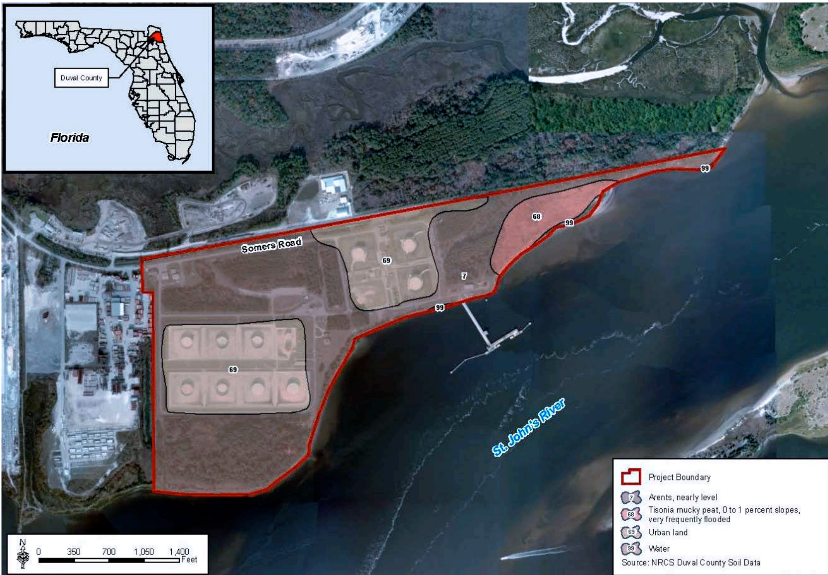
Figure 3-2. Soils Data for Fleet and Industrial Supply Center Jacksonville Navy Fuel Depot (NFD).
