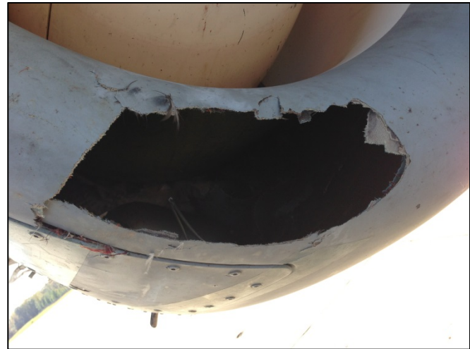
Figure 4-37. Collision with red-tailed hawk on 22-Oct-2012, resulting in destroyed lower intake panel and $29,100 in repair costs
