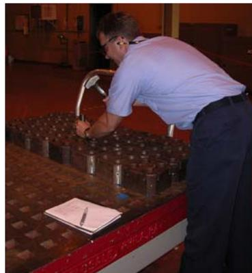
Figure 2: Using a sledge hammer to create a wire junction
