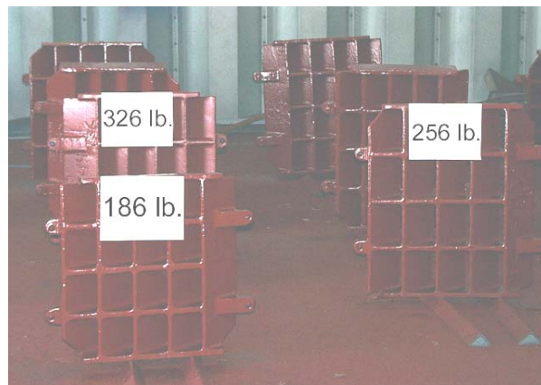
Figure 4: Grates weighing 186, 256, and 326 lbs. in upright position
