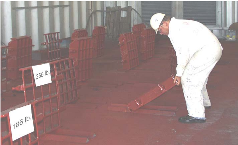
Figure 2: Employee flipping grate. Grates shown weigh 186 and 256 lbs.
