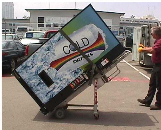
*Use special dollies and other equipment to make lifting easier, faster, and safer.*
