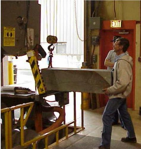
Use hoists or other equipment for lifting to make the job easier, faster, and safer.
