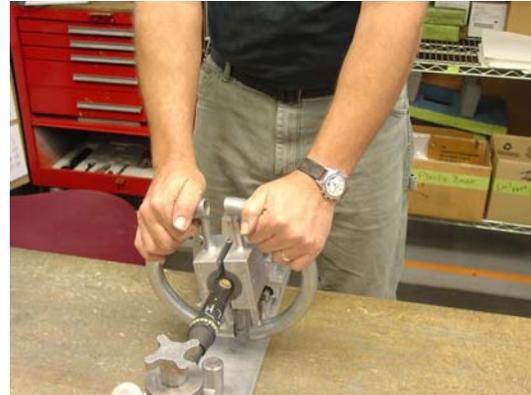
A custom deep socket used with a standard socket wrench allows the operator to use a tool to turn the nuts instead of turning by hand—so easy it can be done with just one finger!
