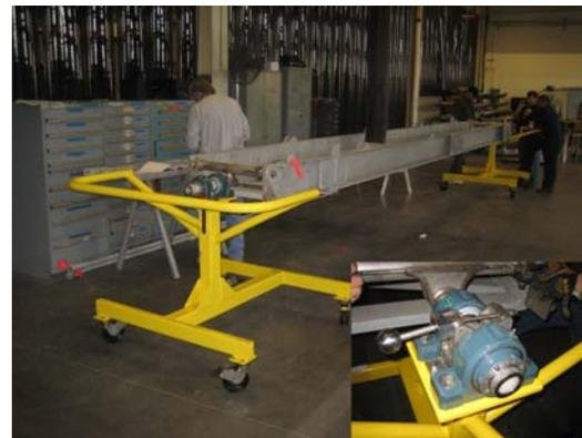
After: Rotating ladder fixture allows one worker to safely turn the ladder and lock it into place. The ladder system saves time and effort, and reduces the risk of injury and equipment damage.
