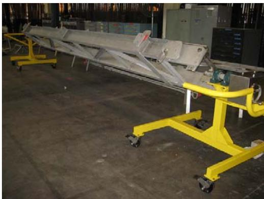
After: Rotating ladder fixture orients easily into the position that best suits the worker and the task whether it be welding or bolt removal, continually fitting the task to the person.
