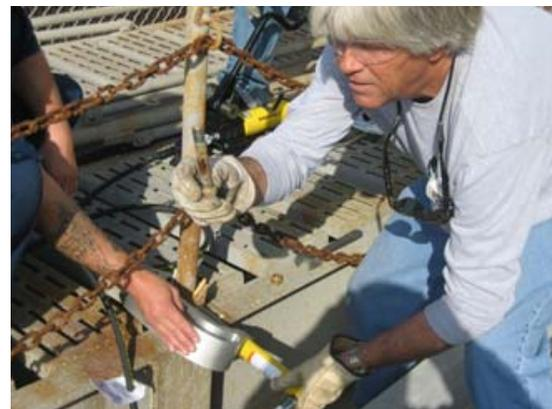
After: The stanchion removal tool effortlessly pushes the bolts free and eliminates the manual method.
