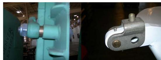
Examples of brass bushing (left) and hinge (right) on a watertight fitting reworked during repair process.
