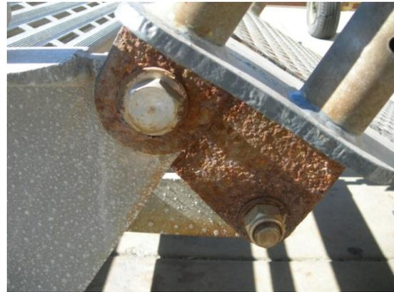
Previously seized bolts/bushings/pins were removed with an impact hammer or by manually hammering them out. Blunt impact, both first aid and lost workday injuries, occurred from the manual method.
