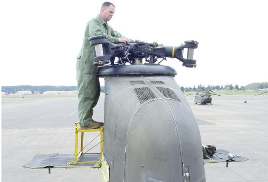
The difference in height seriously reduces fatigue and the possibility of overhead injuries.
