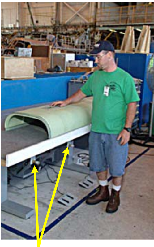
Pneumatic manifold with three couplings. No falling over airlines.
