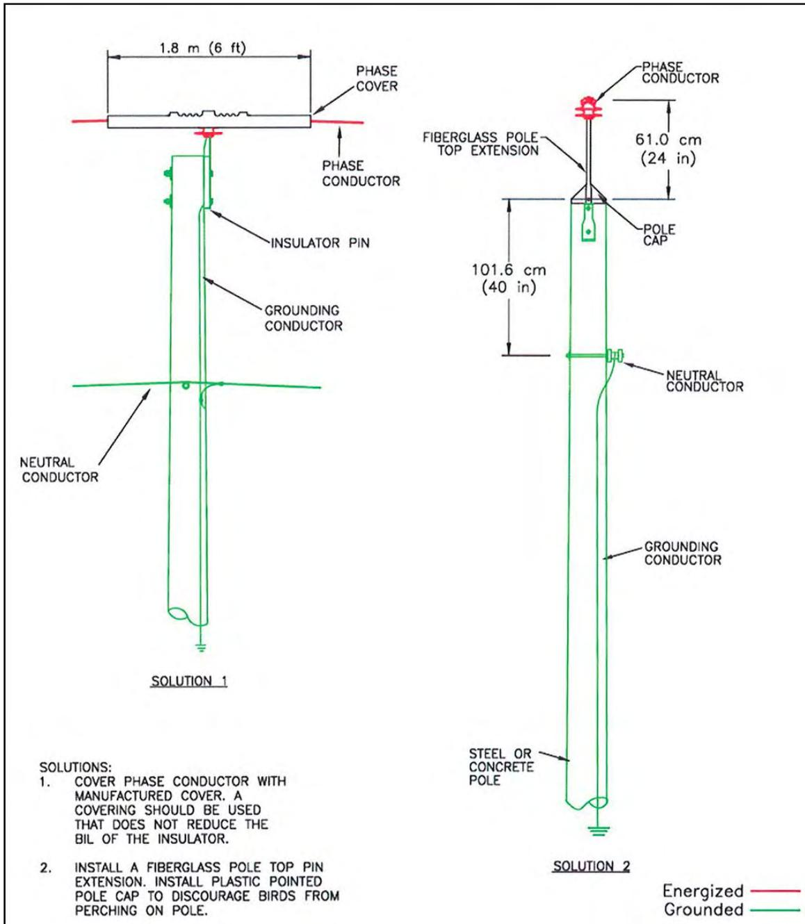
Figure A-23. Solutions for single-phase configuration on a steel or reinforced concrete pole.
