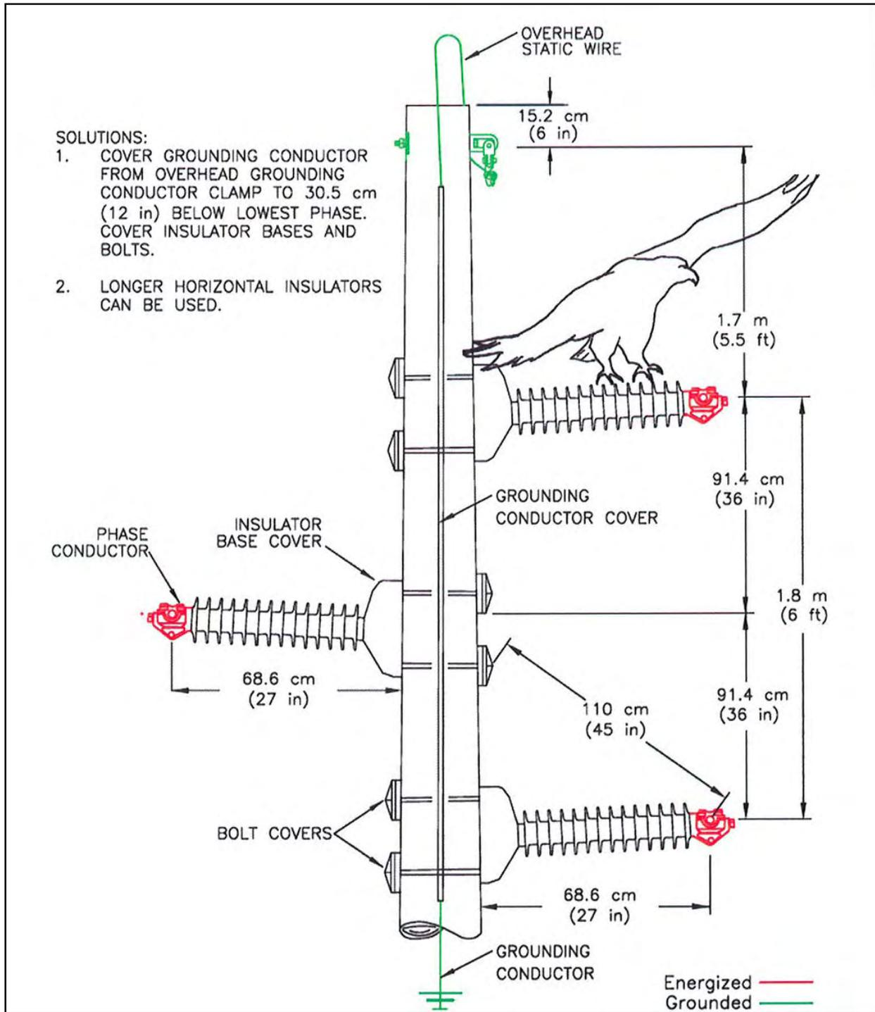
Figure A-30. Solutions for 69-kV horizontal post insulator design.
