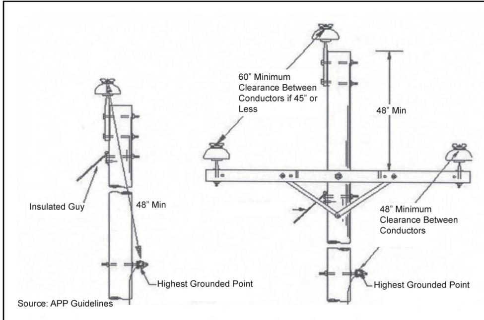
**Figure 11. Avian-safe Structure with Proper Conductor Separation**
