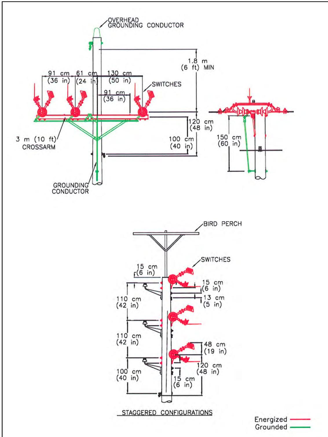
Figure A-44. Pole-mounted switches
