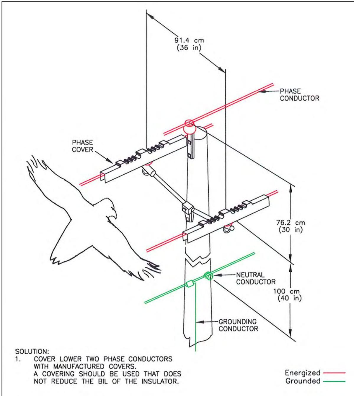
Figure A-13. Solution for compact three-phase design.
