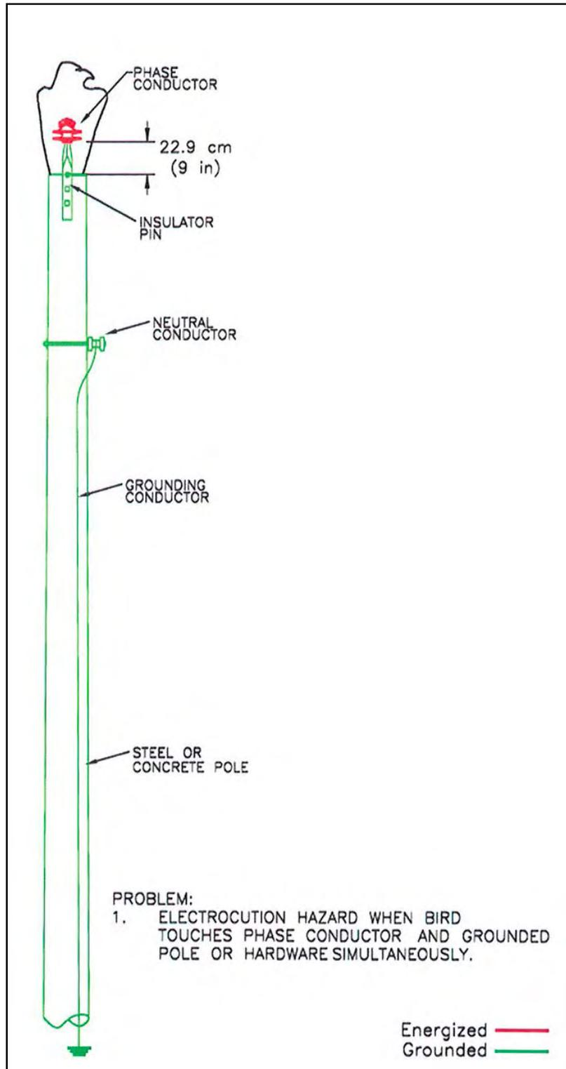
Figure A-22. Problem single-phase configuration on a steel or reinforced concrete pole.
