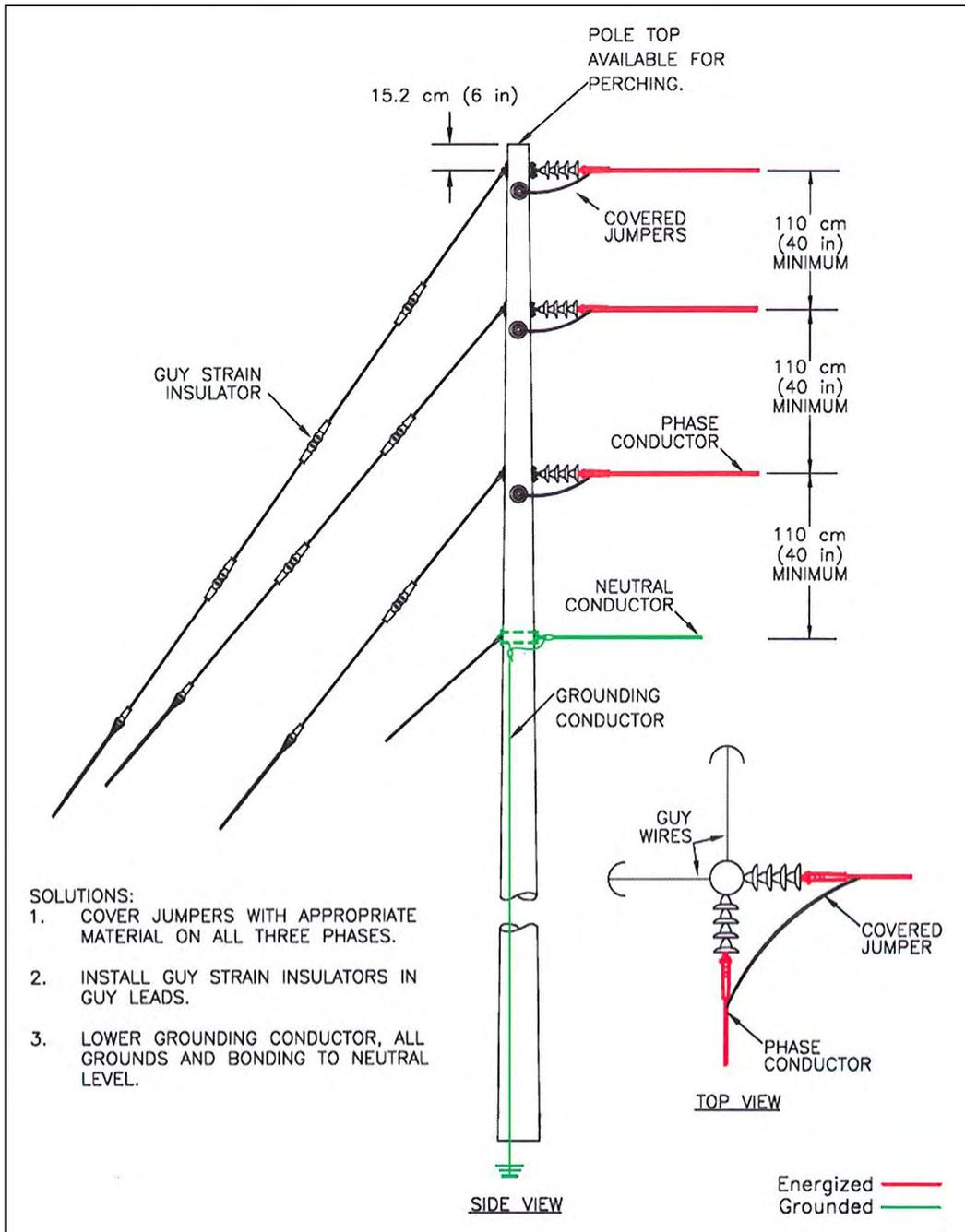
Figure A-20. Three-phase vertical corner configuration—neutral below phases.
