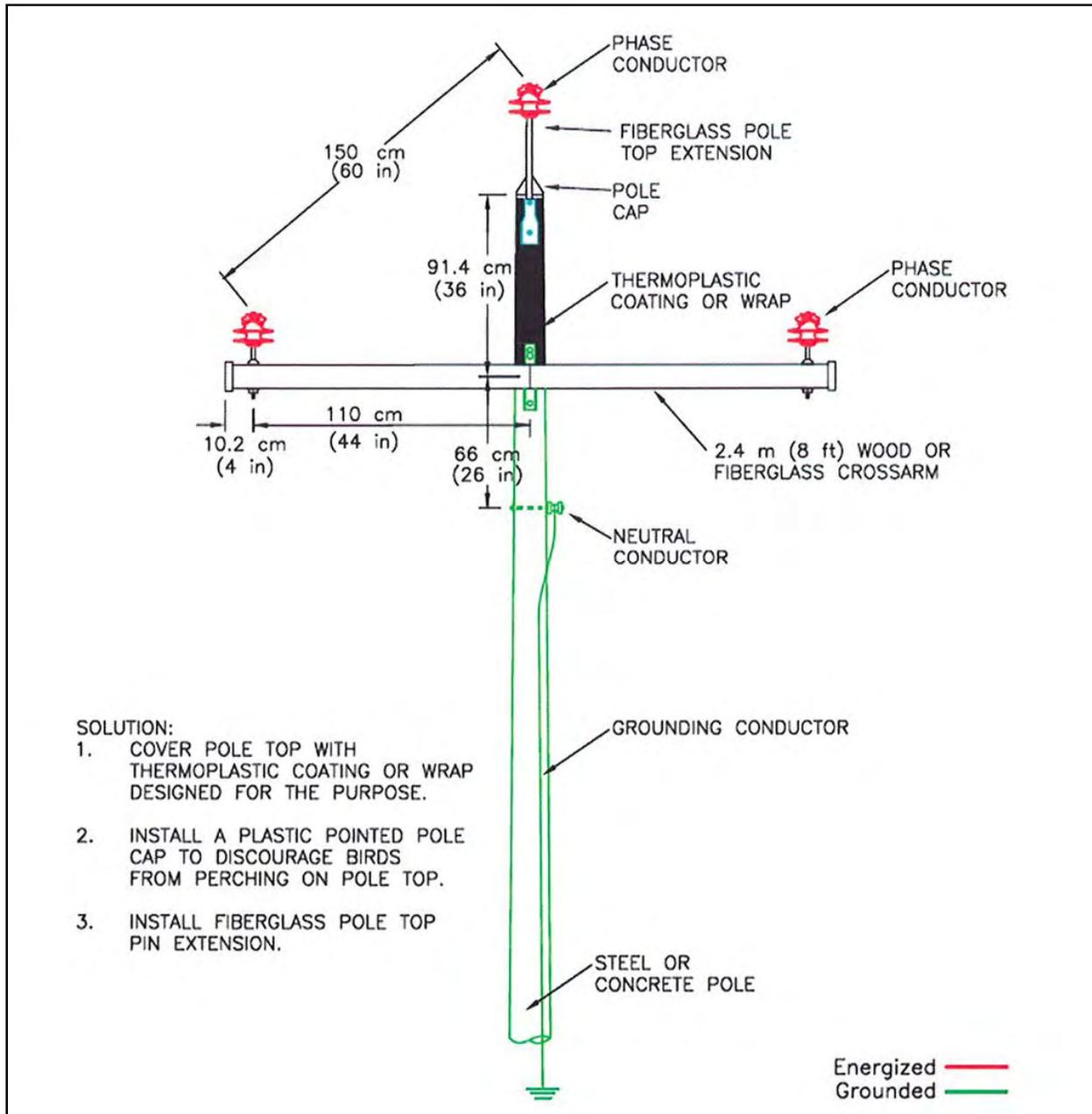
Figure A-25. Solution for three-phase configuration on a steel or reinforced concrete pole using thermoplastic wrap.
