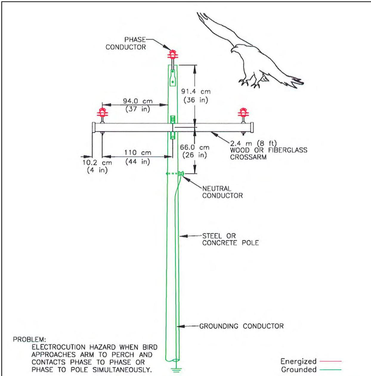
Figure A-24. Problem three-phase configuration on a steel or reinforced concrete pole.
