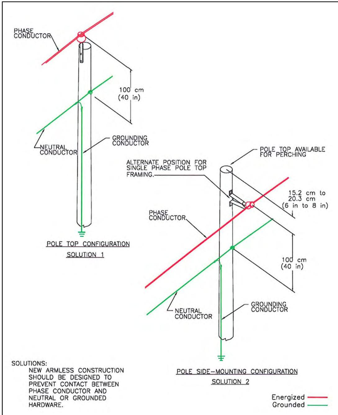
Figure A-5. Single-phase avian-safe new construction.
