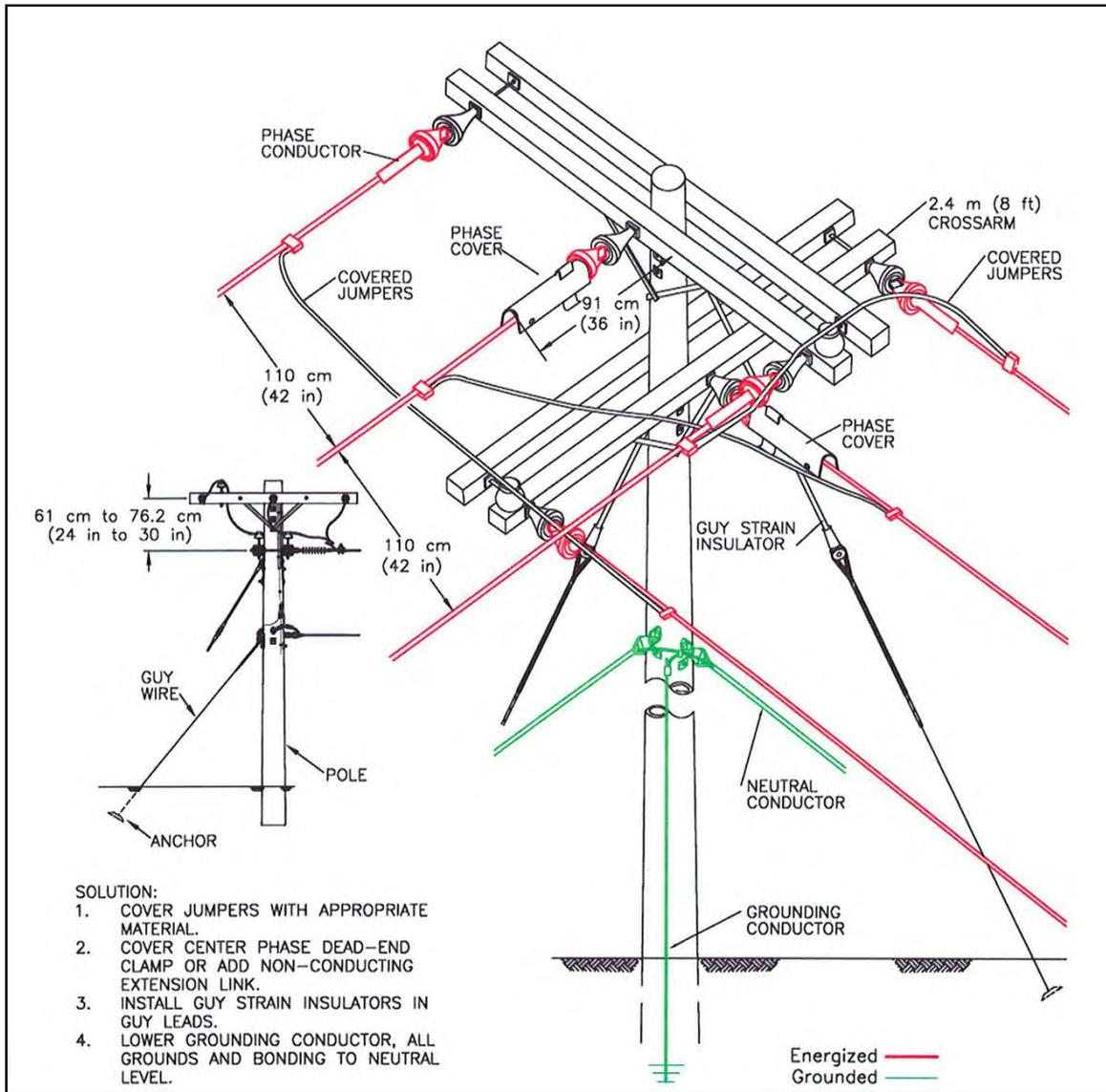
**Figure A-18. Solution for three-phase distribution corner configuration.**
