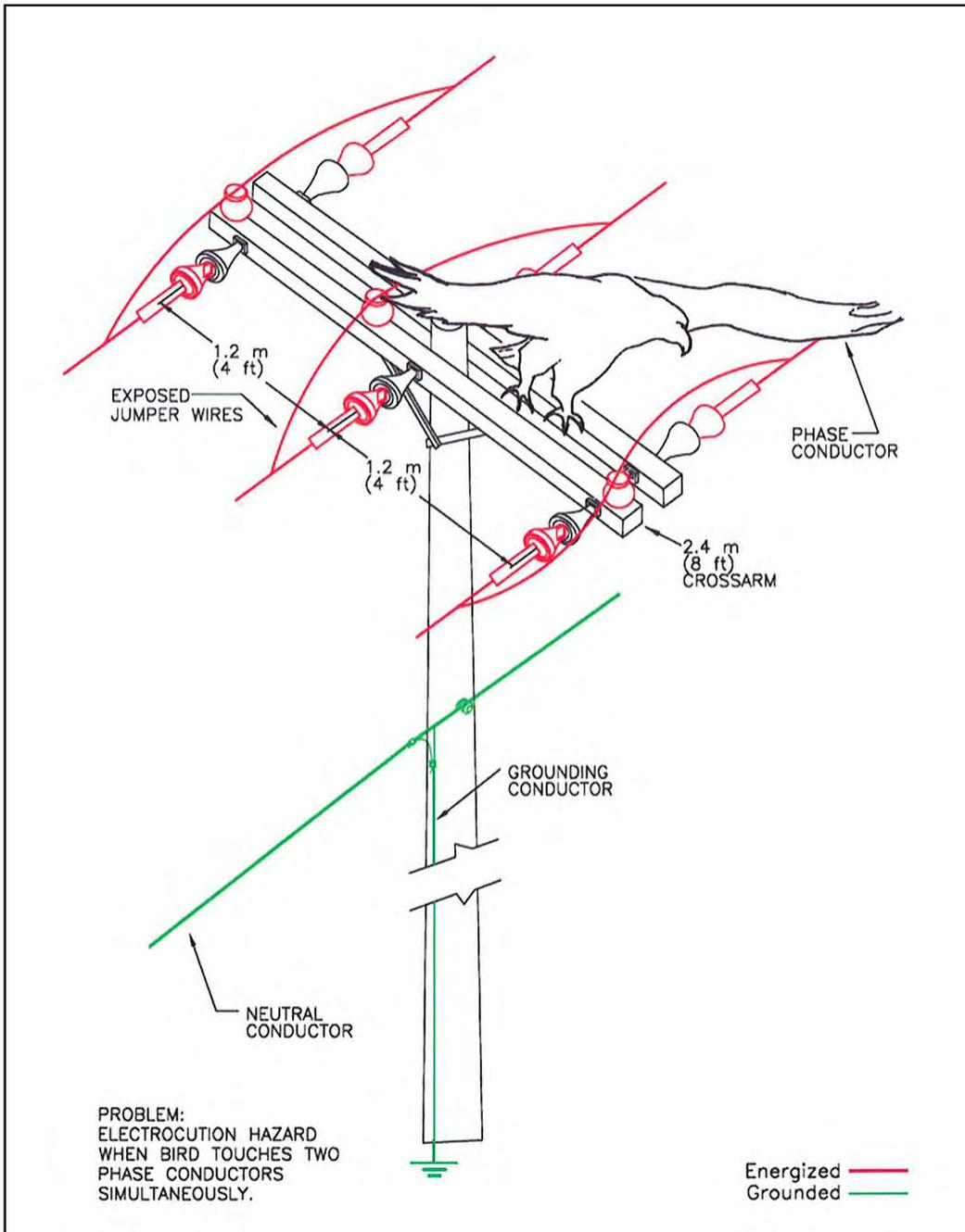
Figure A-10. Problem three-phase double dead-end with exposed jumper wires.
