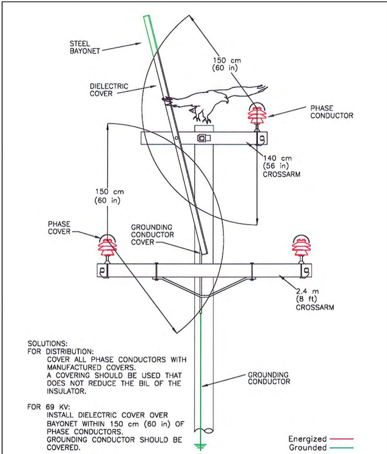
Figure A-36. Solution for design with grounded steel bayonet.
