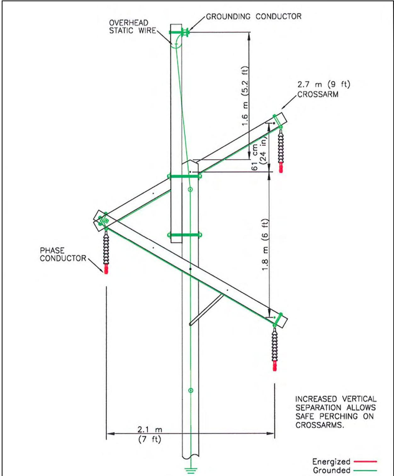
Figure A-33. Avian-safe wishbone construction.
