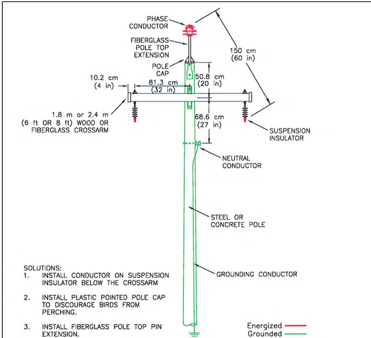
**Figure A-28. Three-phase configuration on a steel or reinforced concrete pole with suspended insulators.**
