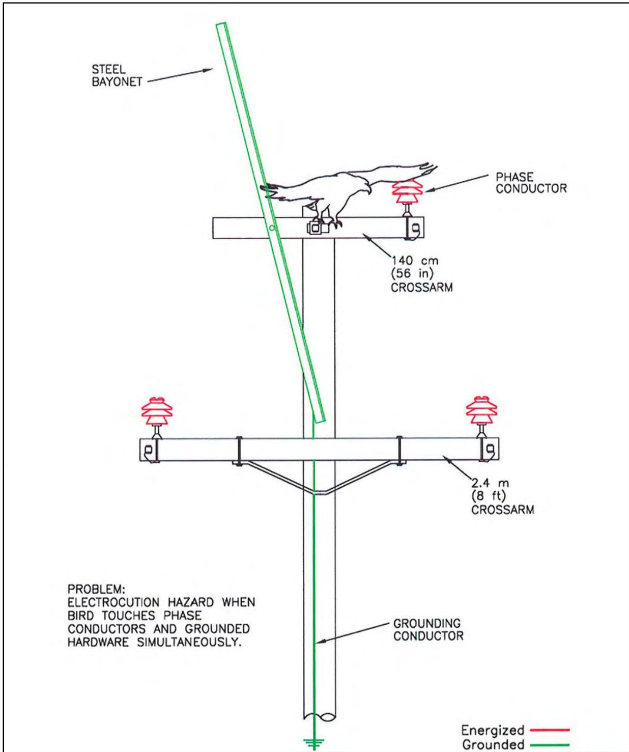
Figure A-35. Problem design with grounded steel bayonet.
