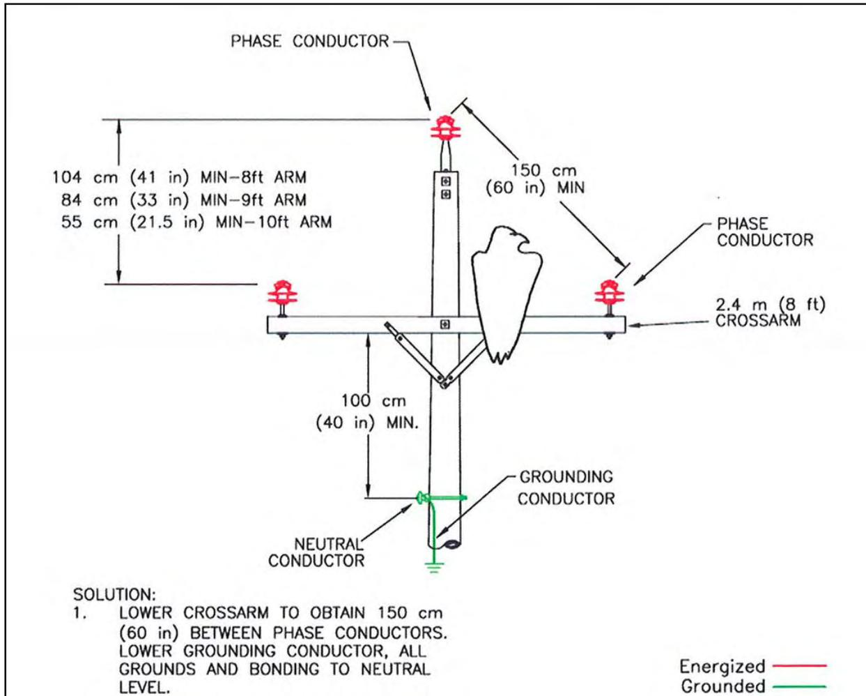
Figure A-8. Avian-safe three-phase construction for different length crossarms.
