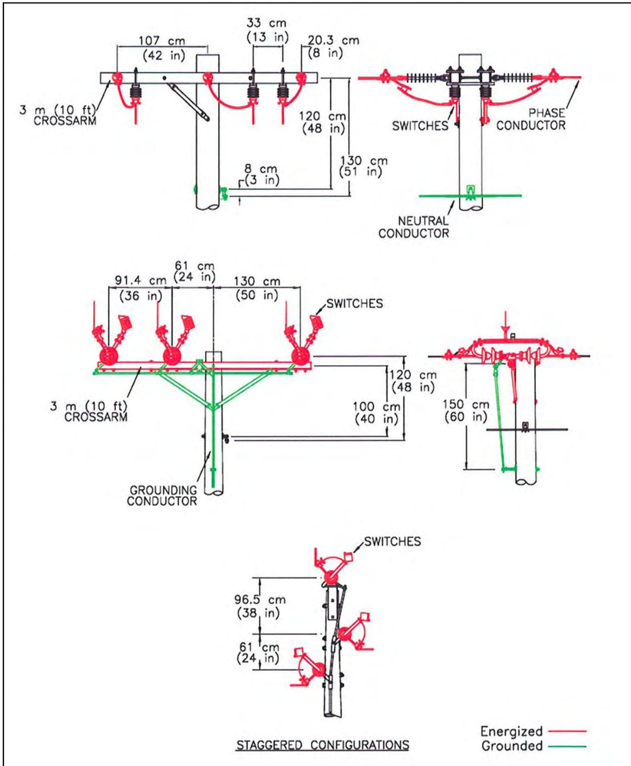
Figure A-43. Pole-mounted switches.
