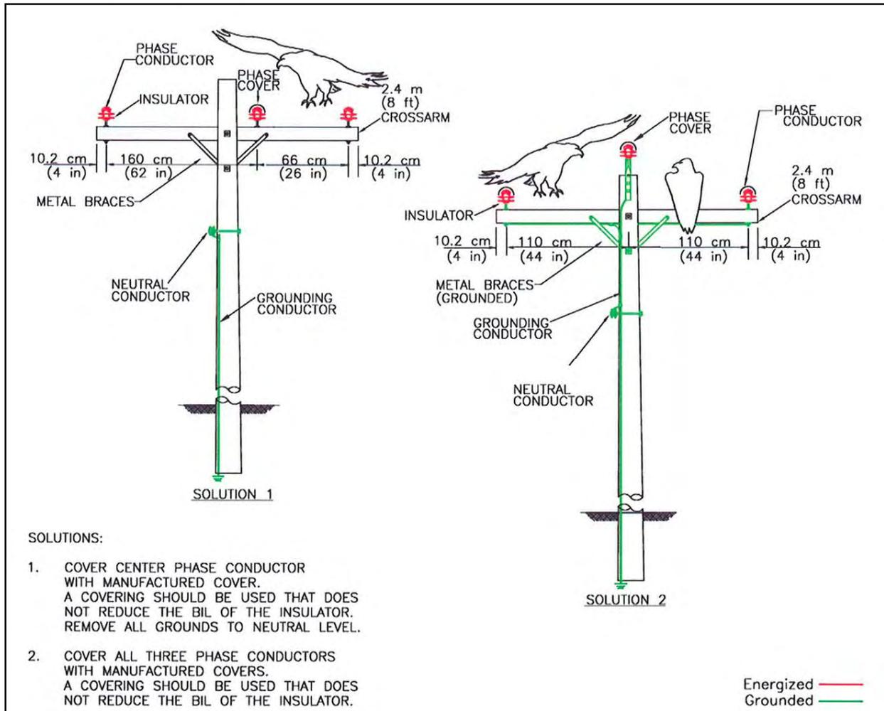
**Figure A-7. Solutions for three-phase crossarm designs with and without grounded hardware.**
