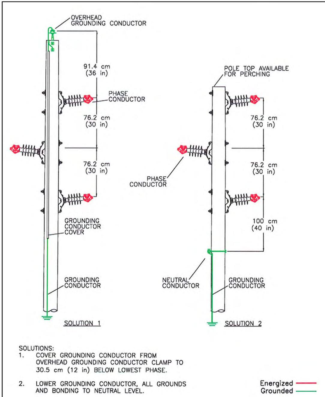
Figure A-16. Solutions for distribution horizontal post insulator designs.
