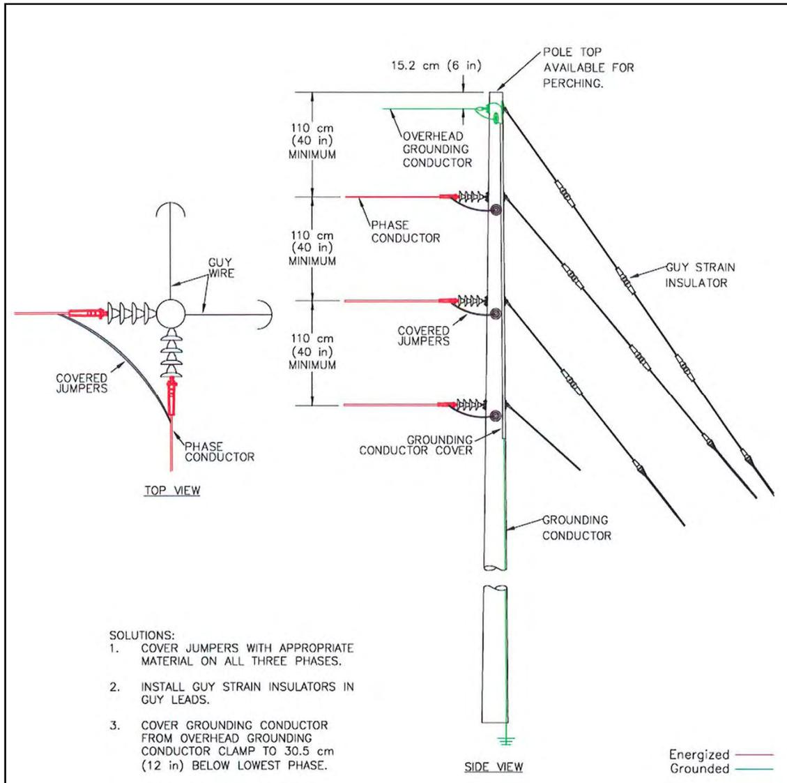
**Figure A-19. Three-phase vertical corner configuration—overhead grounding conductor on pole top.**
