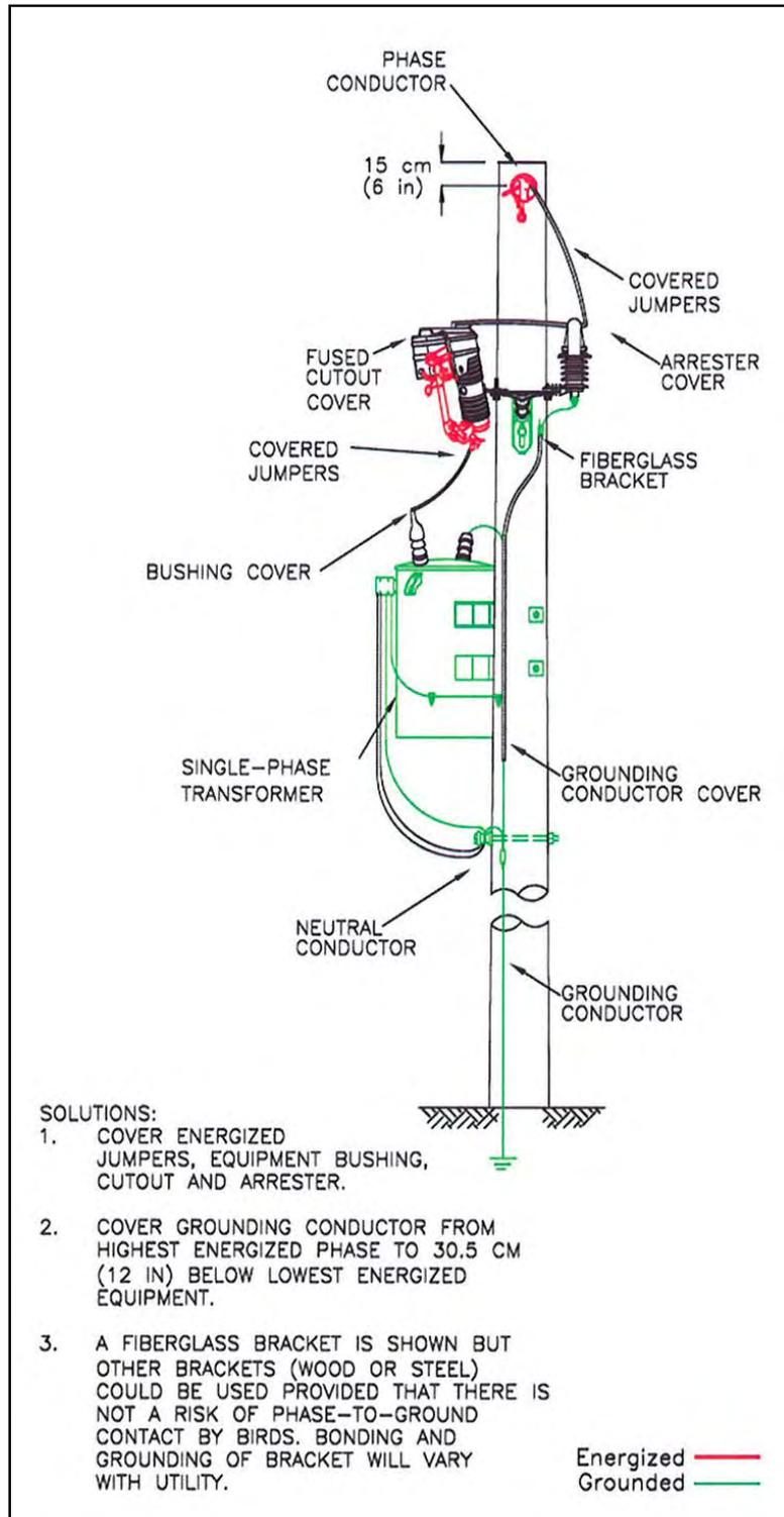
Figure A-42. Solution for single-phase transformer bank.
