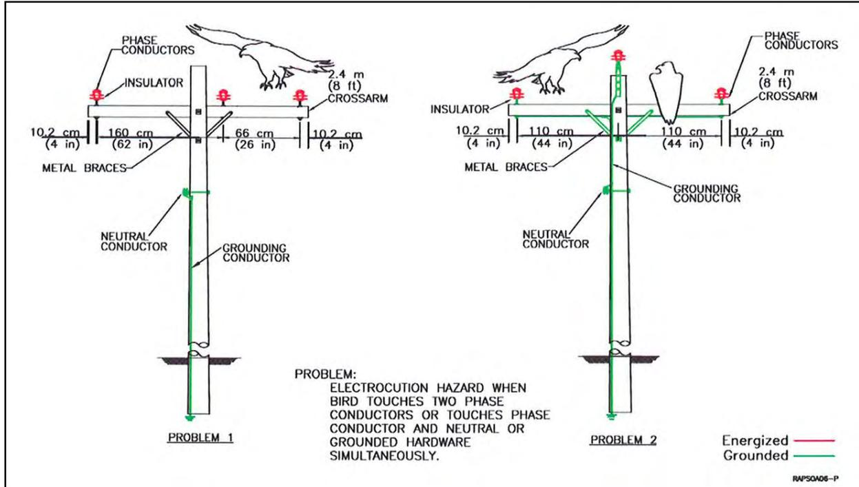
Figure A-6. Problem three-phase crossarm designs with and without grounded hardware.
