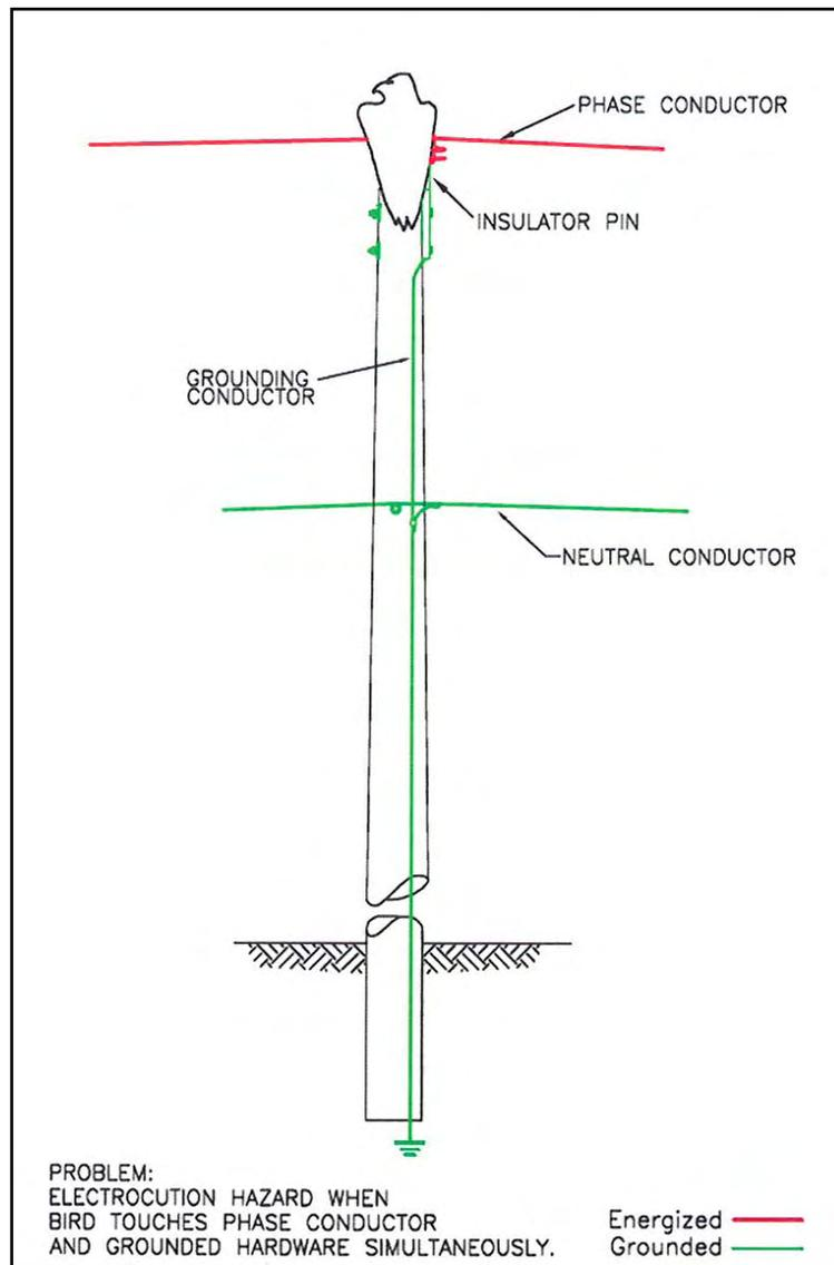
Figure A-1. Problem single-phase with ground pole-top pin.
