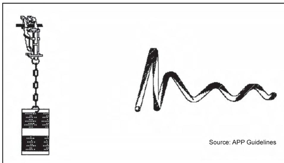
**Figure 23. Swinging Marker Device (Left) and Bird Flight Diverter (Right)**
