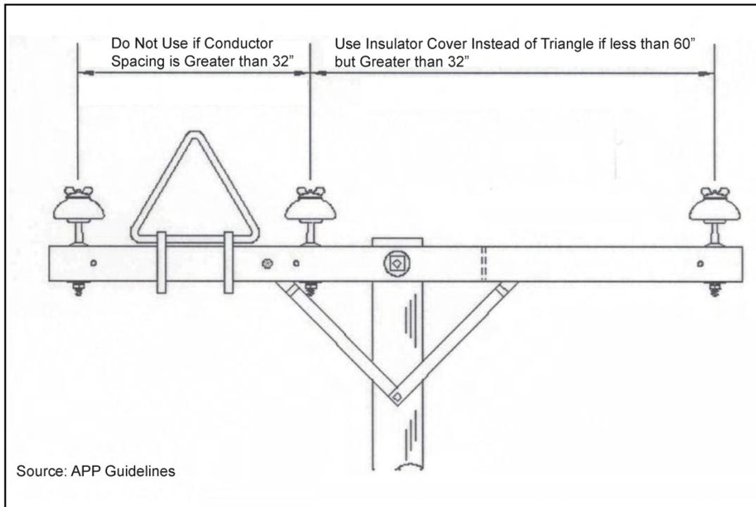
**Figure 20. Avian-safe Structure with Perch Guard**
