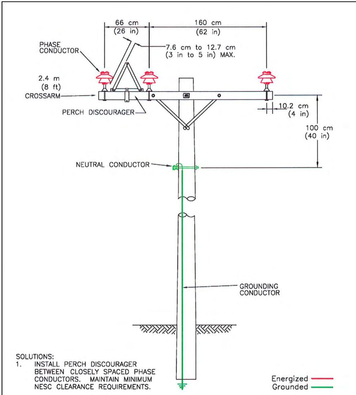
Figure A-9. Solution for three-phase crossarm using perch discourager.
