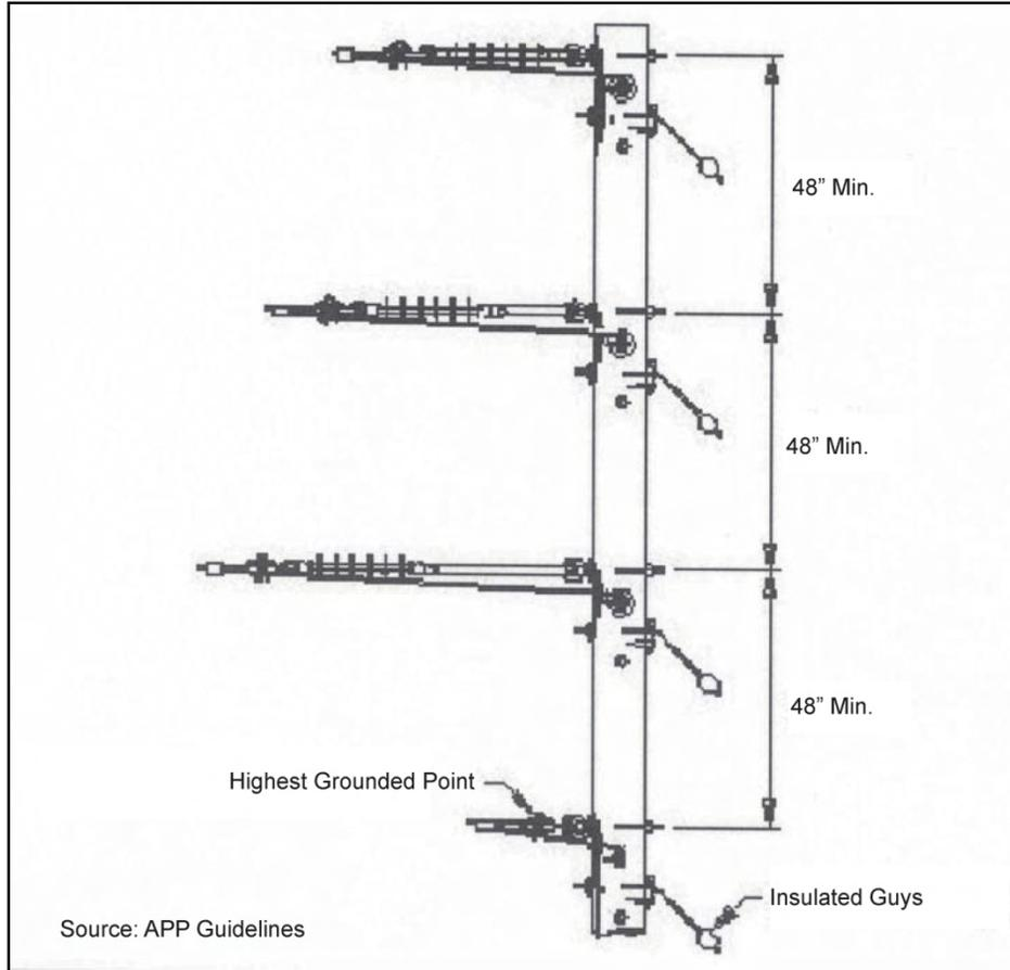
**Figure 13. Avian-safe Structure with Proper Conductor Separation**
