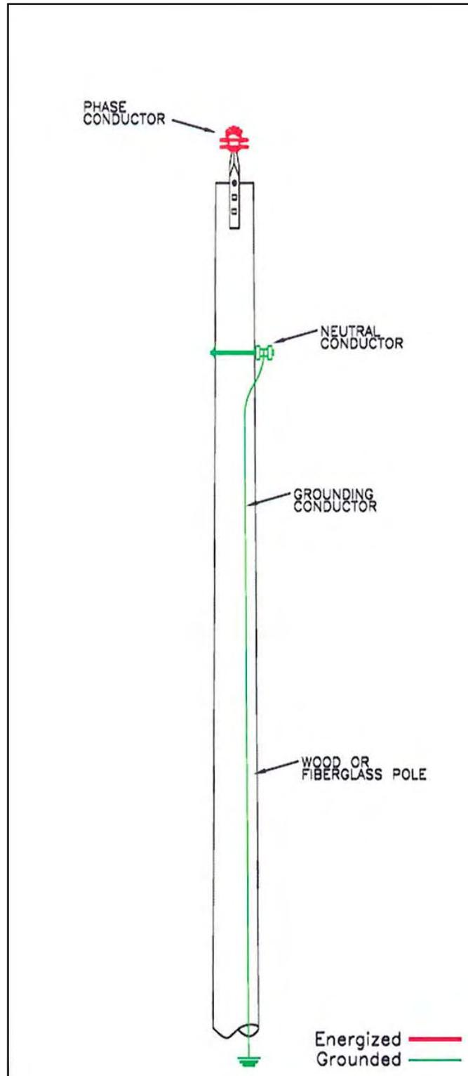
Figure A-21. Typical single-phase distribution configuration on a wood or fiberglass pole.
