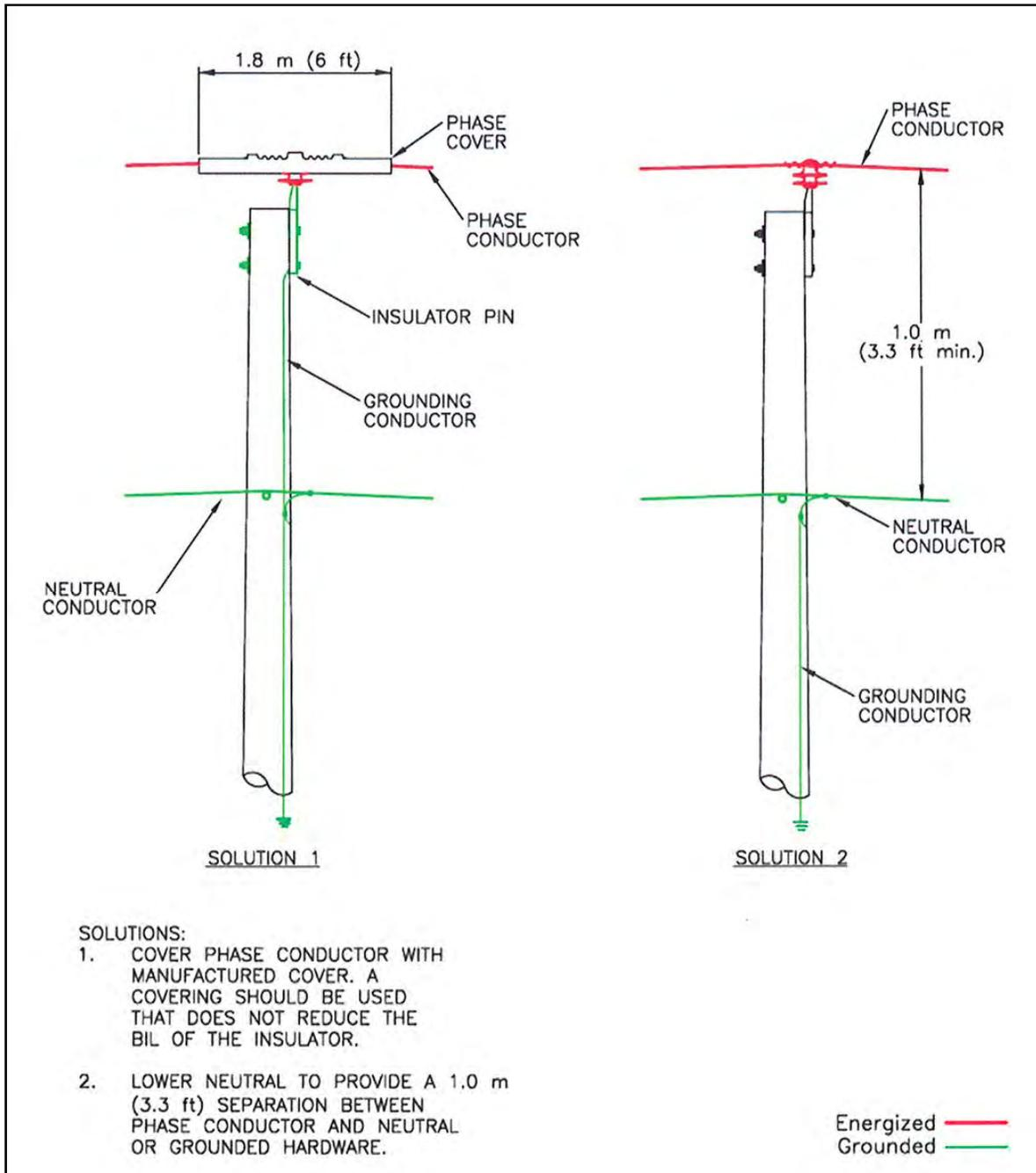
Figure A-2. Solutions for single-phase with ground pole-top pin.
