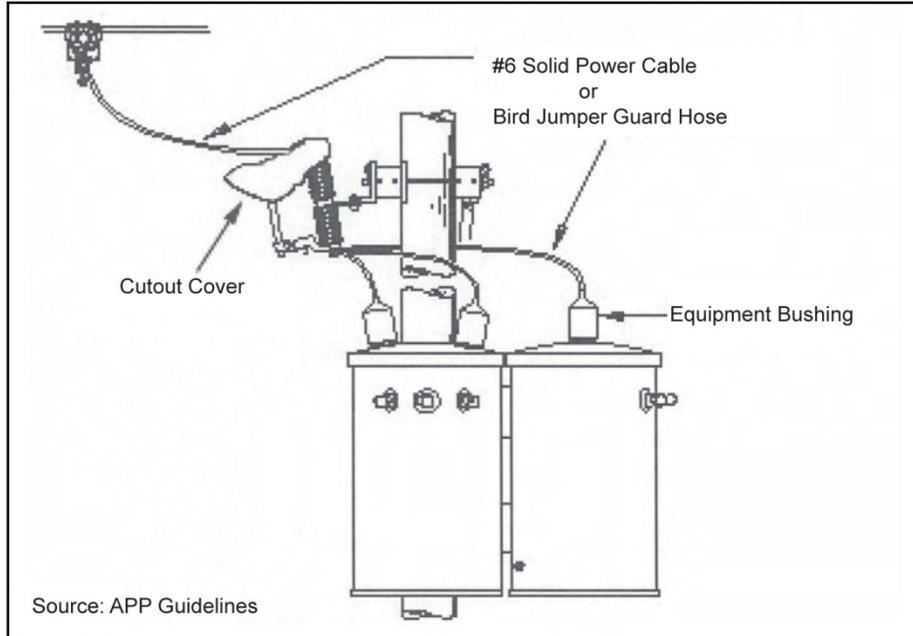
**Figure 16. Avian-safe Structure with Insulated Covers**
