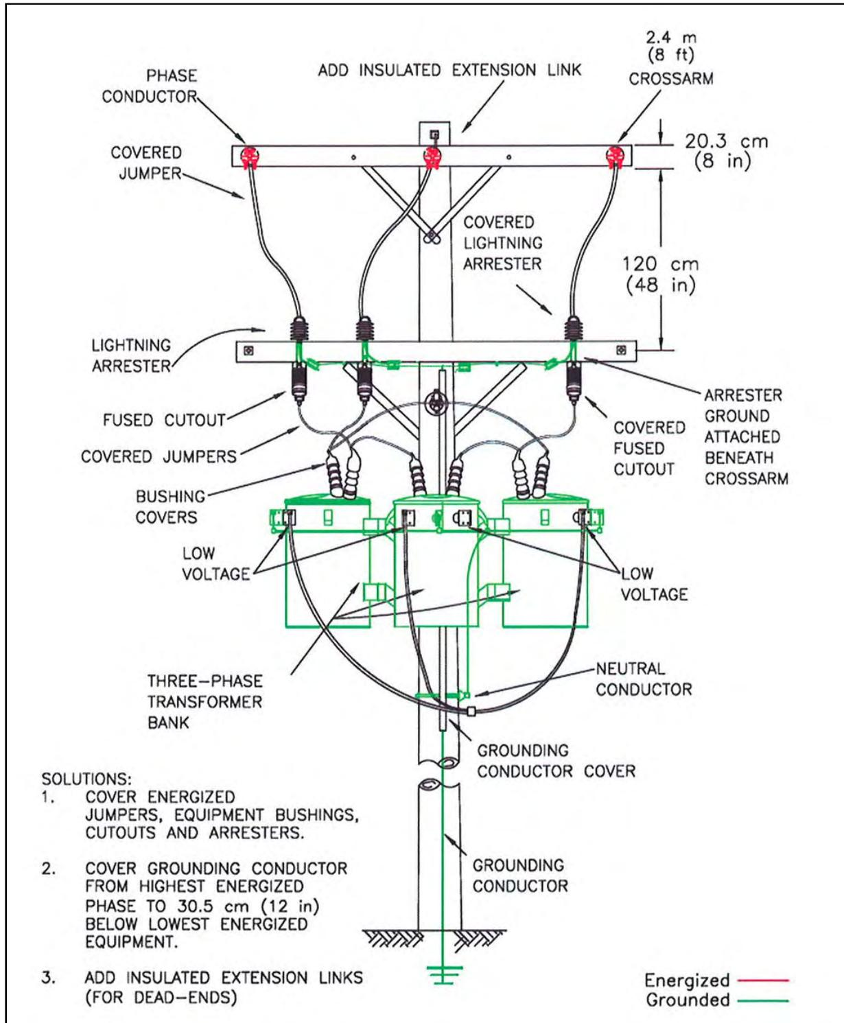
Figure A-41. Solution for three-phase transformer bank.
