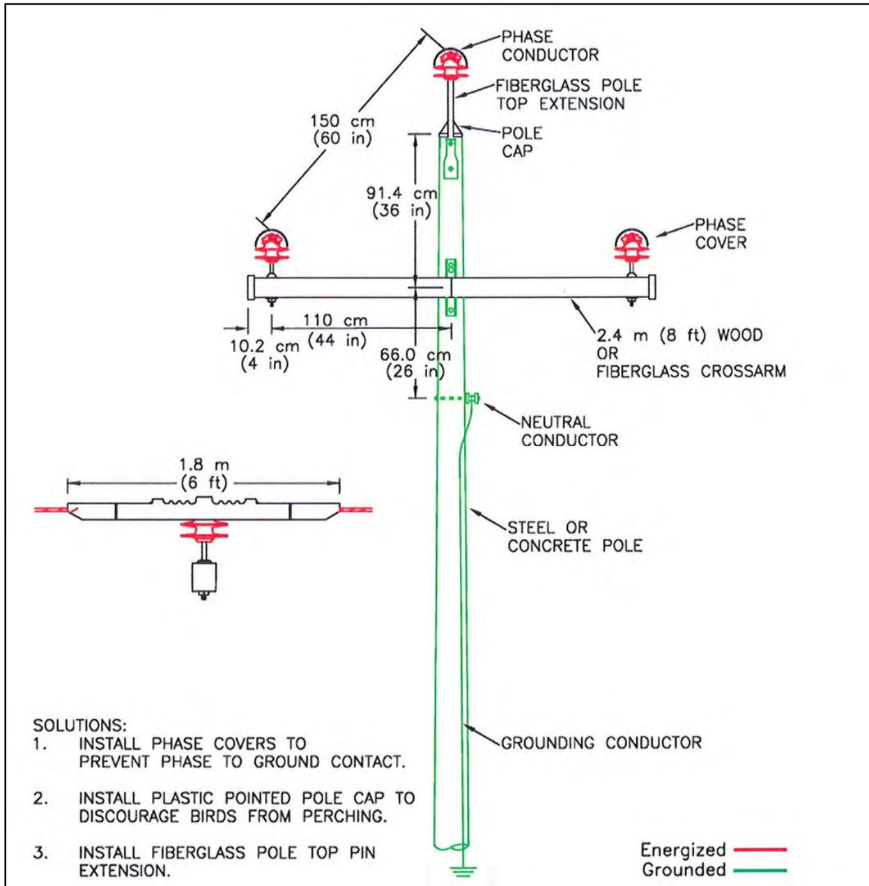
**Figure A-27. Solution for three-phase configuration on a steel or reinforced concrete pole using phase covers.**
