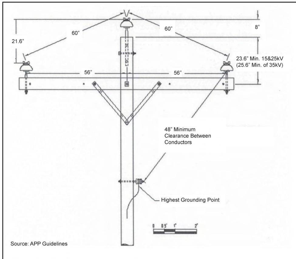
**Figure 12. Avian-safe Structure with Proper Conductor Separation**
