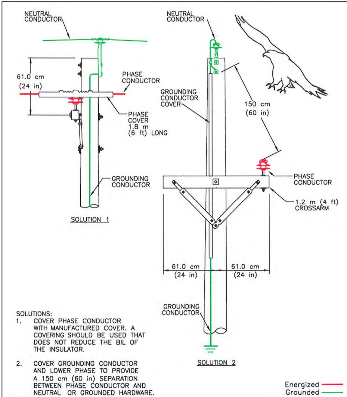
Figure A-4. Solutions for single-phase configuration with crossarm and overhead neutral.
