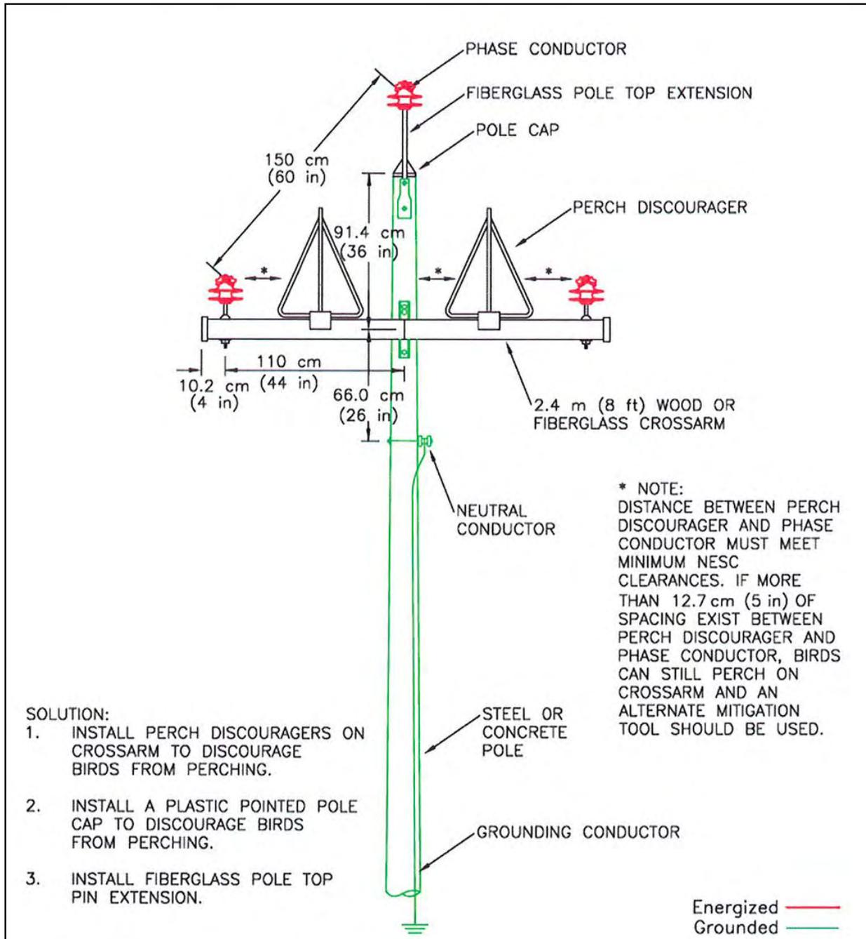
Figure A-26. Solution for three-phase configuration on a steel or reinforced concrete pole using perch discouragers.
