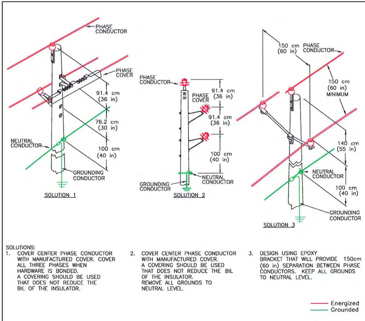
Figure A-14. Avian-safe compact three-phase designs for new construction.
