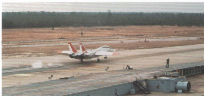
A different sort of "bird" tests a catapult launch at the Navy Lakehurst research facility./Naval Air Engineering Center
