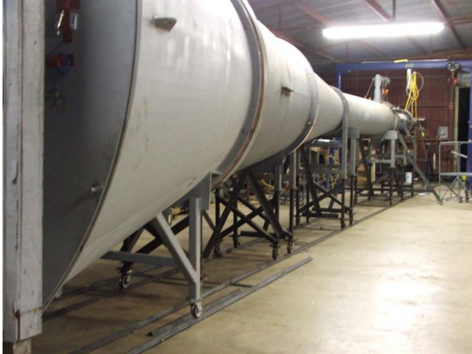
**Figure 2. ABS Consulting Shock Tube Apparatus**
