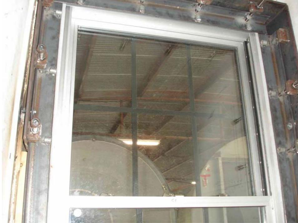
**Figure 3. Steel Sub-frame with Window Mounted in Test Cubicle**
